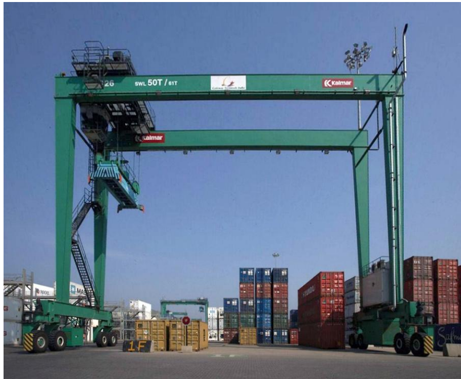
Figure 9 Rubber Tire Gantry Crane (RTG)
