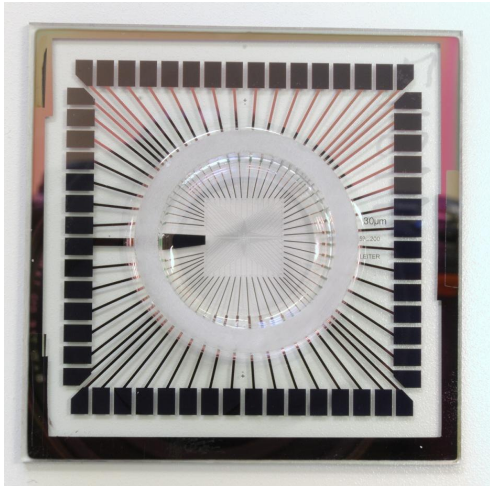
Figure 3.7. Typical MEA dish. The microelectrode area is located in the middle of the dish, and the large electrode to left of the array acts as the ground and reference electrode.
