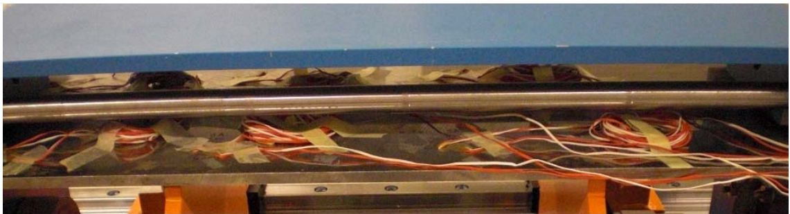
Figure 7.16 Longitudinally strain gages on the guiding walls.
