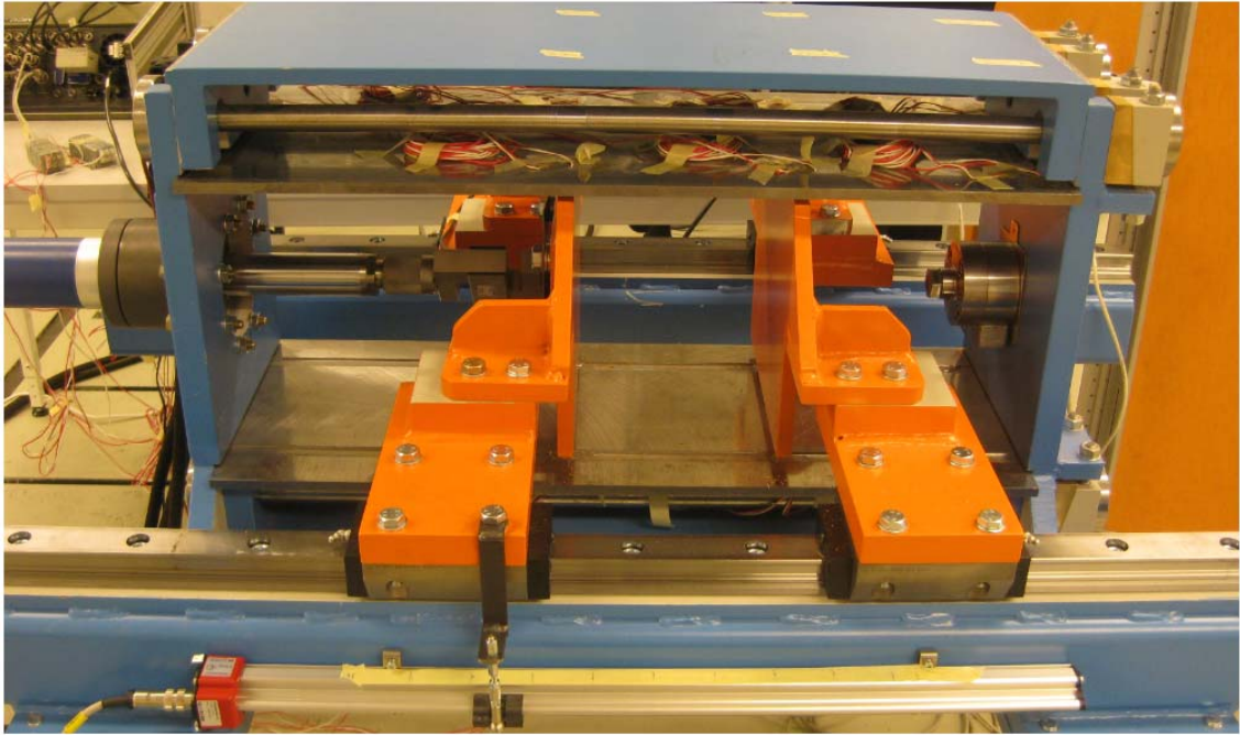
Figure 7.15 Pushing and stop plate force sensors assembly on the unit.
