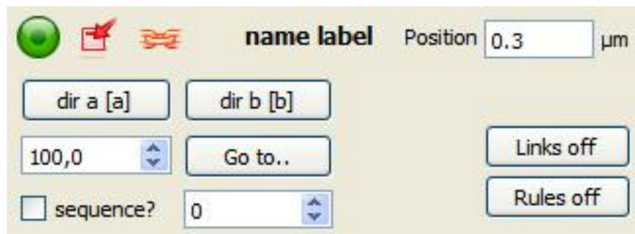
Figure 6.18 MiCo GUI component for closed-loop controlled SmarAct micropositioners
