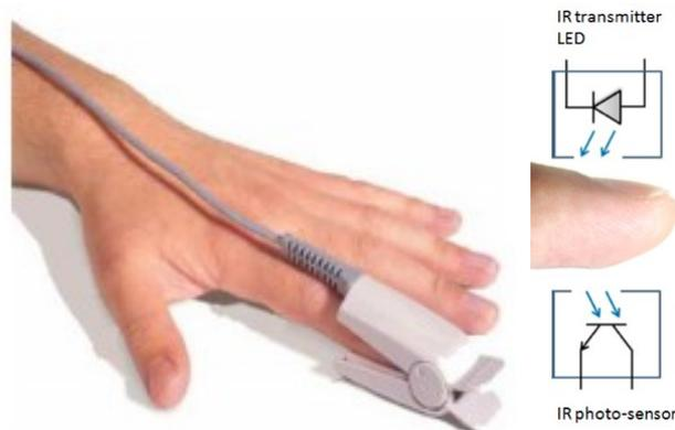
**Figure 12.** An example of a PPG finger clip sensor, which is using infrared light.
