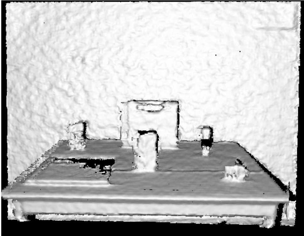
Figure 4. Results of Kinect Fusion's colorless model taken from a single location.
