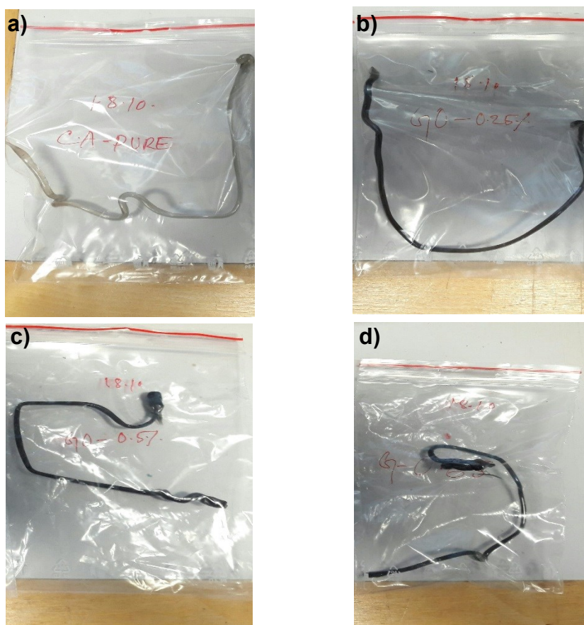
Figure 20. Processed Samples- TEC plasticized a) CA, b) GO 0.25, c) GO 0.50 and d) GO 0.65 Composite samples.
