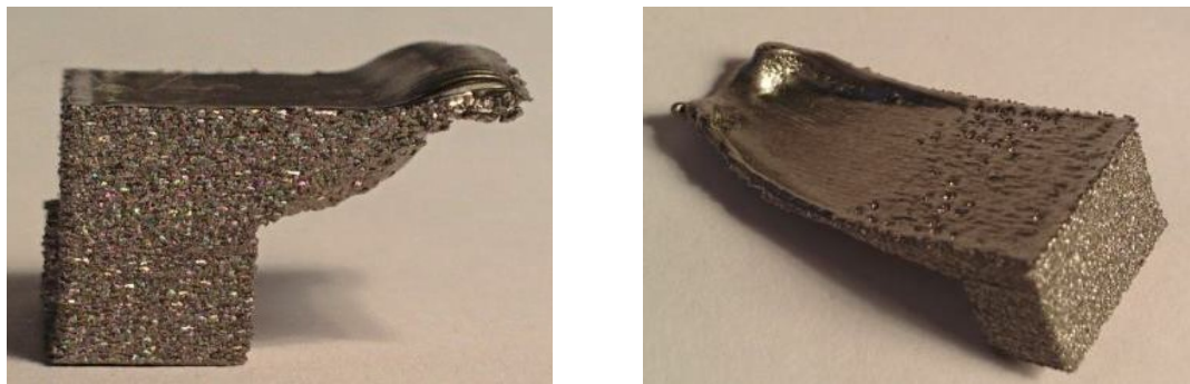
Figure 6. Curling defect in overhanging parts (Tounsi & Vignat, 2017)
