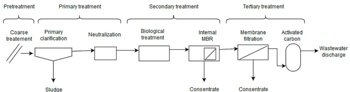
**Figure 4.** Flowchart of pulp mill's wastewater treatment, which contains integrated membrane filtration system, adapted from (Biermann 1996, pp. 287, 289; De Wever *et al.* 2007).
