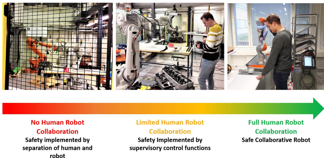
Figure 4. The concept of Human Robot Collaboration.
