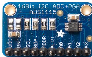
**Figure 4.5** The ADS1115 is a high-resolution ADC converter used in the testbed for purposes to read the generated voltage at the harvester, and to communicate this data (as bits) with the microcontroller.
