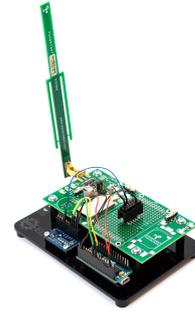
(b) Final receiver structure with attached antenna
