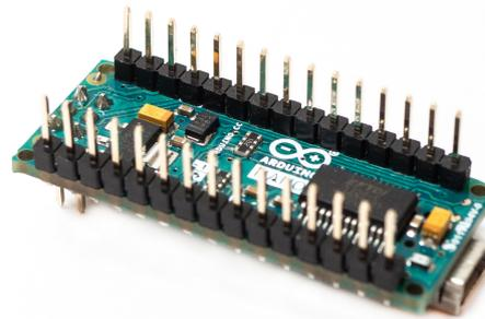
**Figure 4.6** *Arduino Nano used in the testbed implementation. It has similar performance as the broadly used Arduino UNO, with a ATmega328 microcontroller. The device is selected due to its small size and good performance in the acquisition and communication with the computer.*
