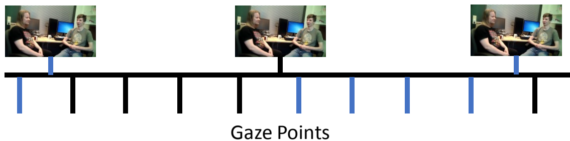
Figure 5.1. Timeline of frames and gaze points arriving with coloring on which frame each gaze point will be mapped.
