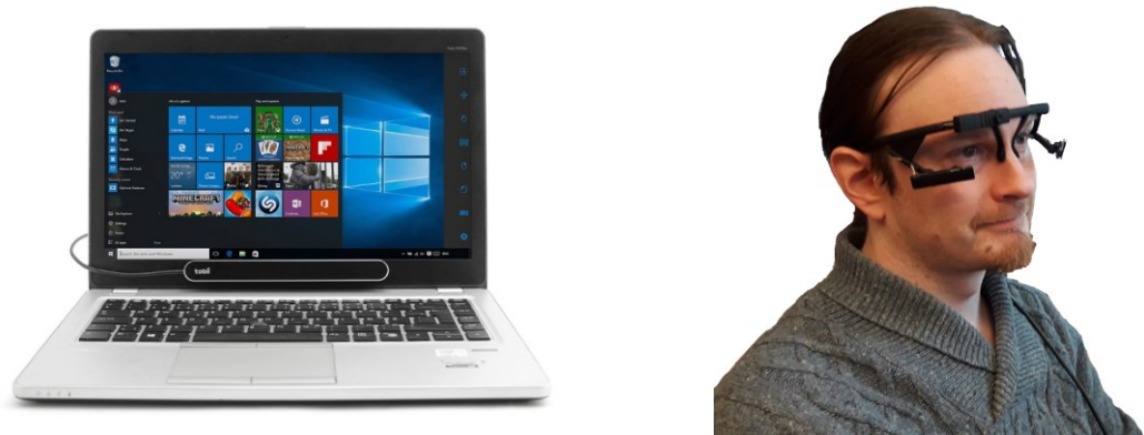
Figure 2.5. A separate eye tracking sensor attached to a laptop [41] and a person wearing eye tracking glasses.
