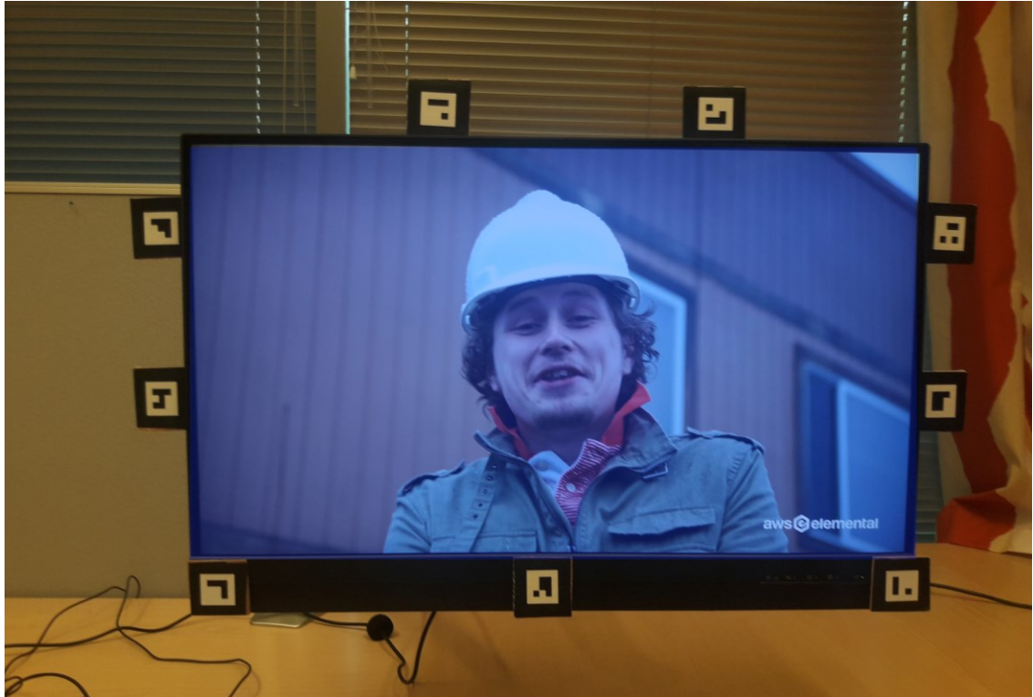
Figure 4.1. The screen with the tags used for tracking.
