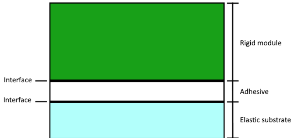
Figure 11. Conceptual joint of a module and substrate.
