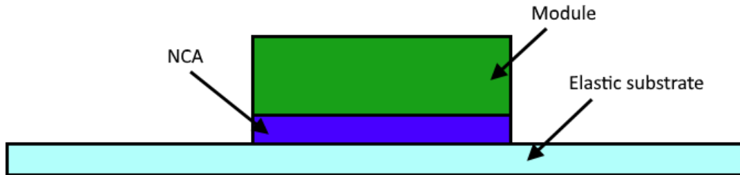
Figure 16. An attached rigid module on elastic substrate.
