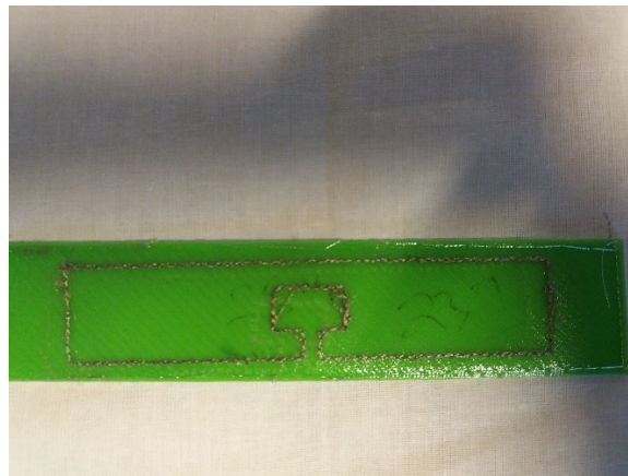
Figure 5-4: Substrate mounted on a white cloth and embroidered
