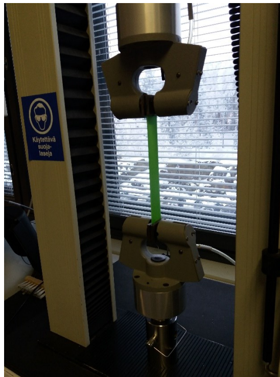
Figure 6-1: Substrate setup on the Instron 4411 Tensile testing machine
