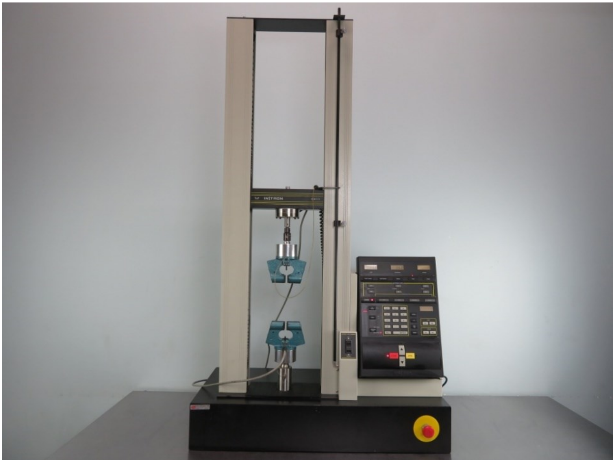
Figure 5-9: Instron 4411 Tensile Strength Tester [44]
