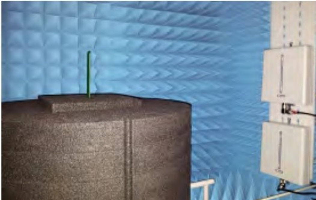
Figure 5-8: Inside view the Tagformance Pro's cabinet [43]
