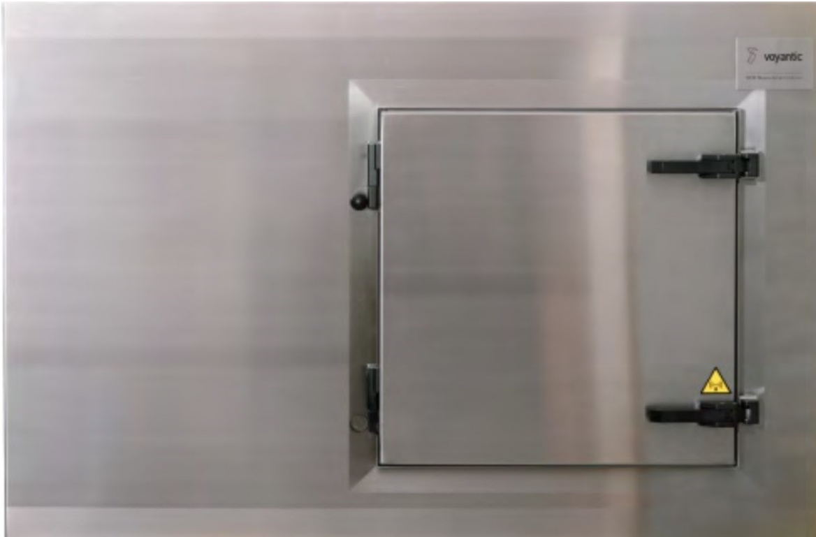
Figure 5-7: The Tagformance Pro's test cabinet [43]
