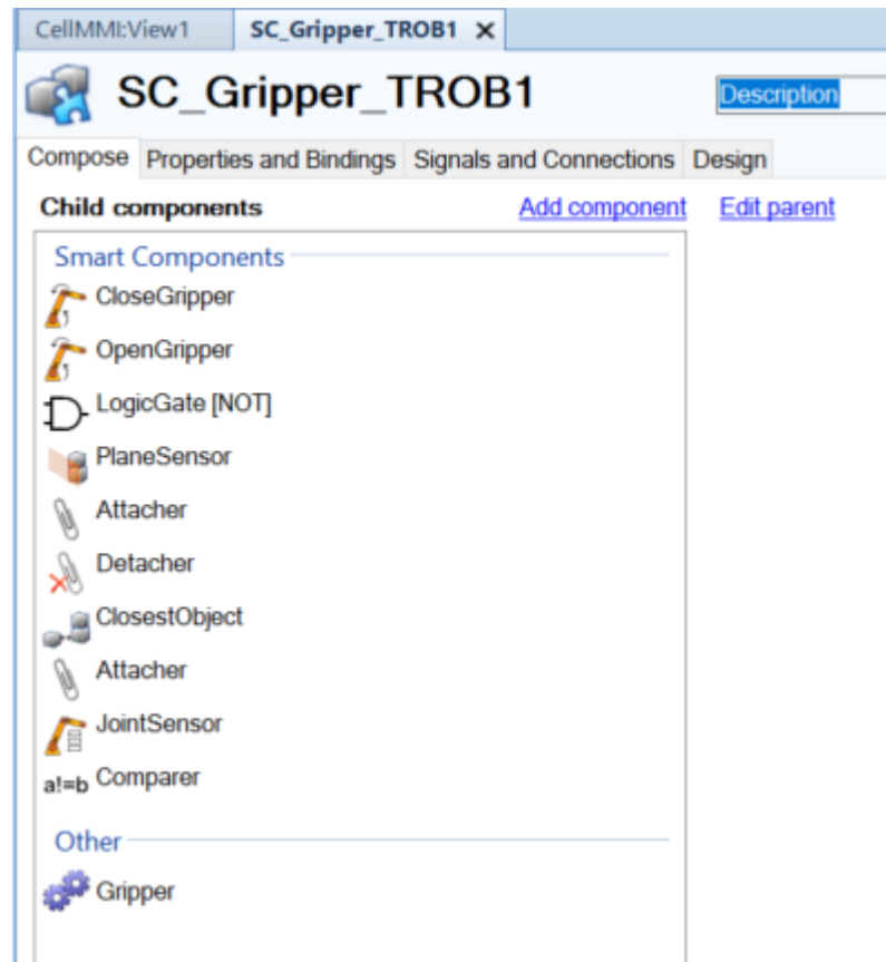
Figure 4.6 Gripper child components. Each of these components works as a function block in the Smart Component design, it also includes the gripper mechanism.
