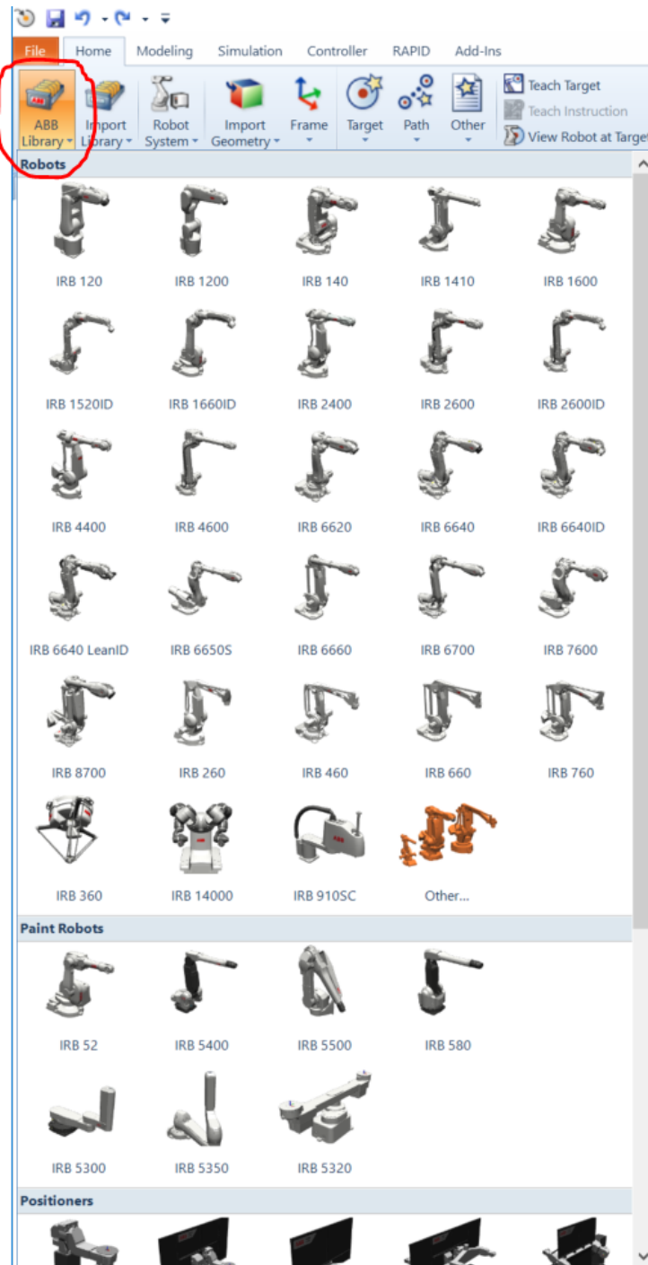
Figure 4.4 How to add robots to the station, using the RS GUI and their library.
