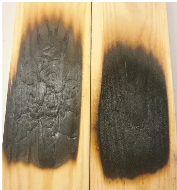
Figure 55. Samples of FR-TC (left) and FR-R2 (right) after the blow torch burning. Thin intumescent layer was formed on the surface of FR-R2 sample.
