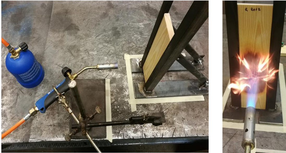
Figure 28. Left: the test setup for the blow torch testing. Right: the blow torch flame on a fire retarded wood surface.
