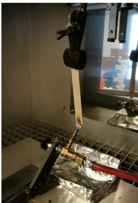
Figure 27. The test setup for the in-house UL 94 test. The small flame cabin and the two centimeter flame was used. A clamp was used to attach the sample to the cabin's frame holder.
