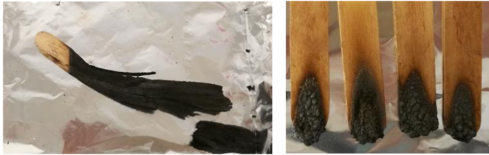
Figure 54. Remains of tongue depressors protected with FR-TC (left) and FR-R2 (right) after the in-house UL 94 burning. Intumescent layer was formed on the FR-R2 samples.
