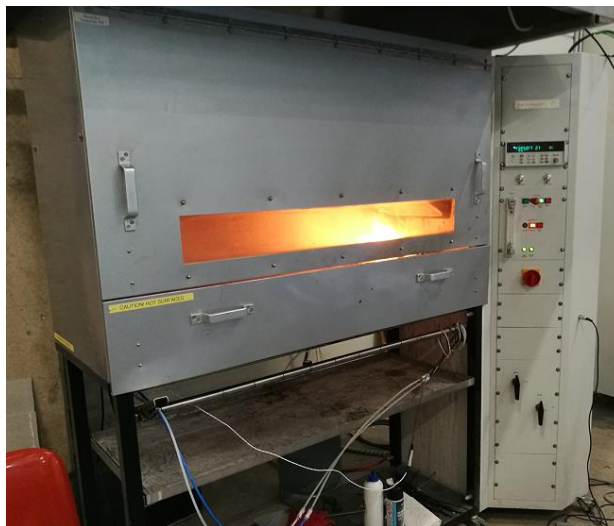
Figure 30. Radiant panel test equipment. A reference sample is burning inside the cabin.
