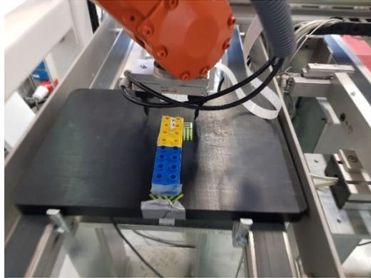
*Figure 33. Workpiece and gripper arrangement for vertical orientation.*
