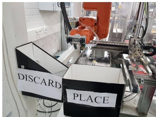
*Figure 40. Place and discard position of the robot.*
