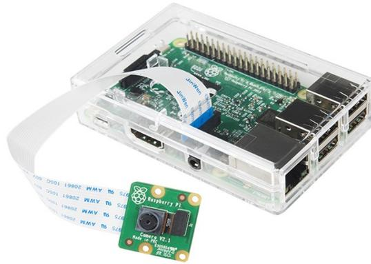
*Figure 22. Raspberry Pi camera module.*
