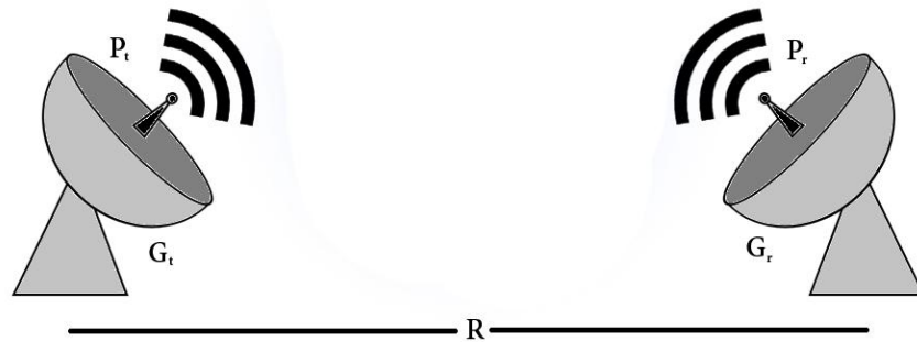
Figure 2-7 Setup for the Friis formula
