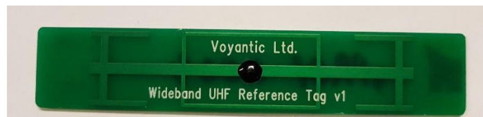
Figure 8-5 Voyantic Ltd. Wideband UHF Reference Tag v1
