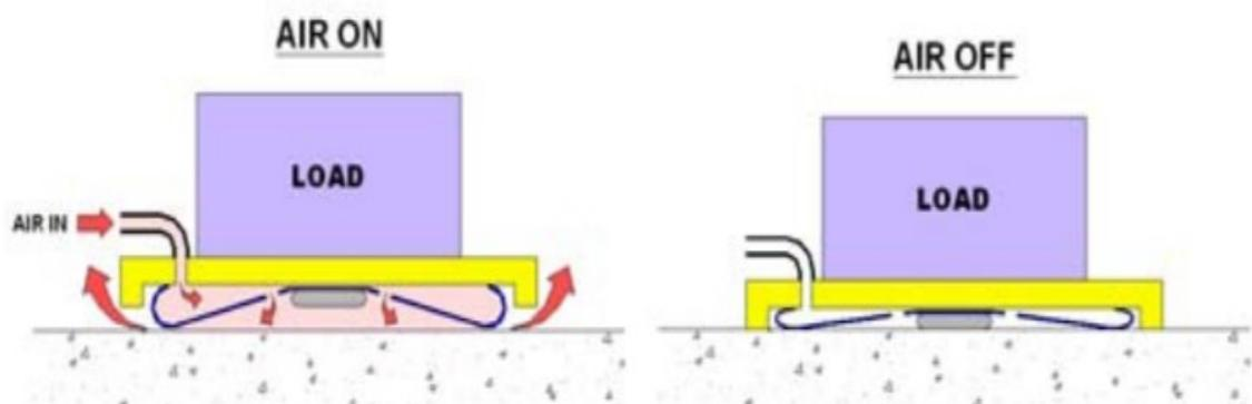
**Figure 2.** On the left an air mover with the air flow on and on the right without the air flow [3]
