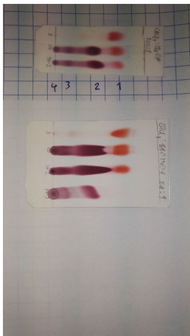
Figure 30. TLC plates used to determine suitable stationary phase/eluent combination. TLC was developed using starting material, co-spot and product, which had been CC purified before.
