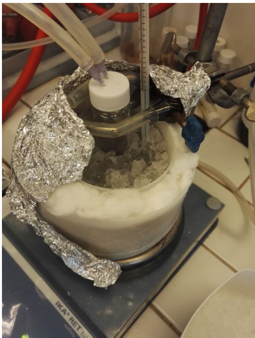
Figure 29. The setup for chilled reaction.
