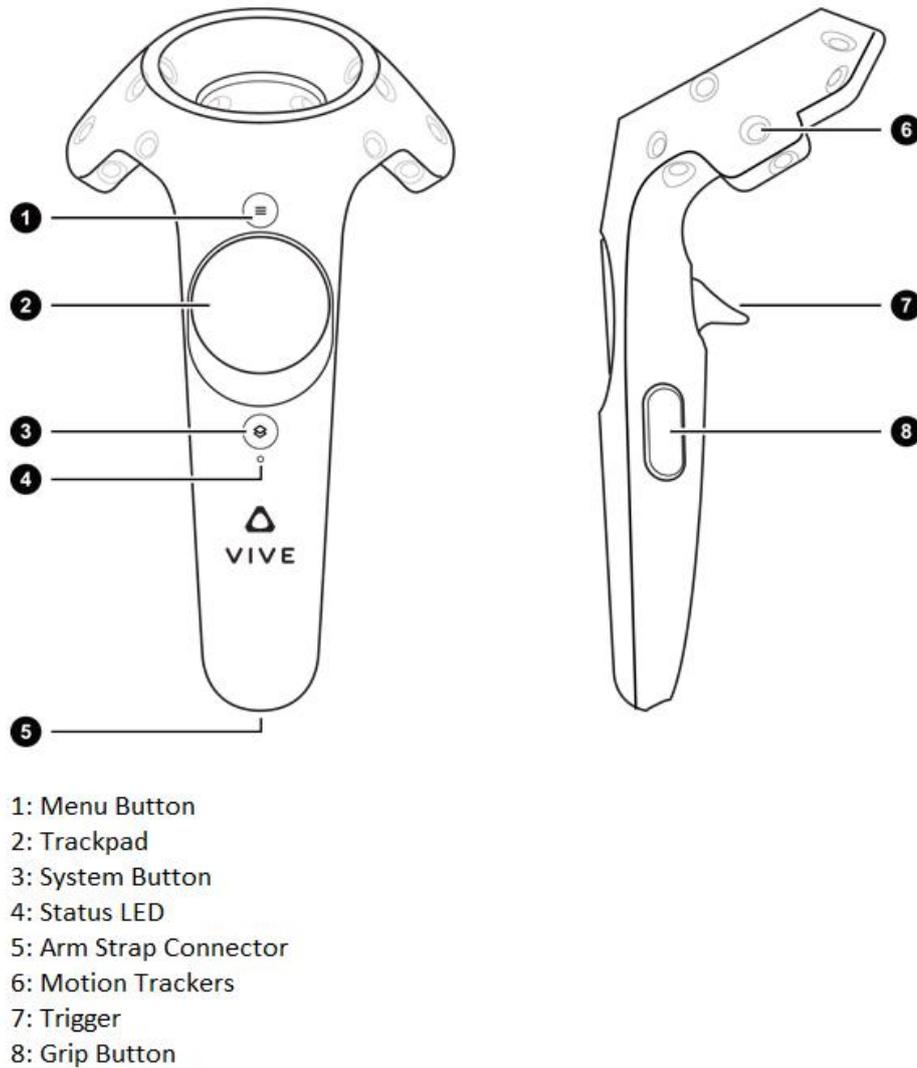
**Figure 27: HTC Vive's controller (Unity Technologies, 2017)**
