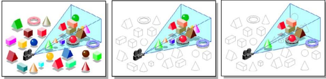
**Figure 15: Illustration of culling. No culling (left), frustum culling (middle), occlusion culling (right) (Johanson, 2016)**
