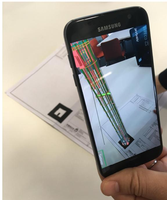
***Figure 4: Example of marker-based AR. The rebar of a column are visualized via mobile device. The QR-Code acts as a marker for the AR software***
