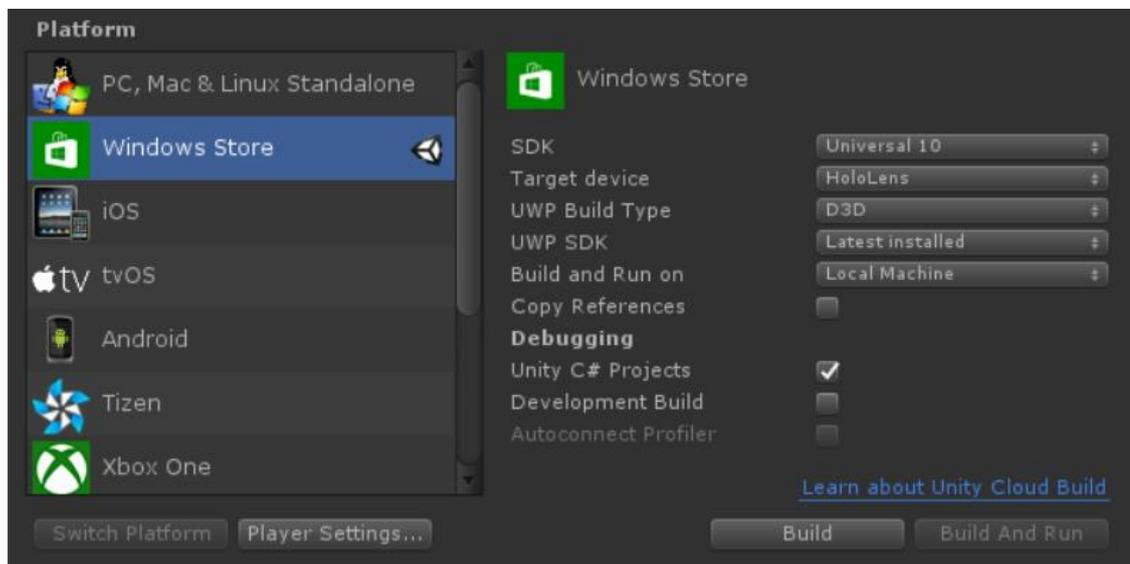
***Figure 32: Unity3D editor's build settings for HoloLens application***
