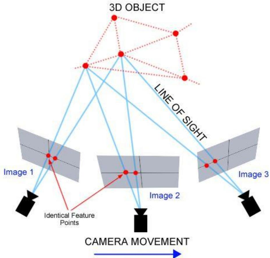
**Figure 6: The basic principle of photogrammetry (Mason, 2016)**
