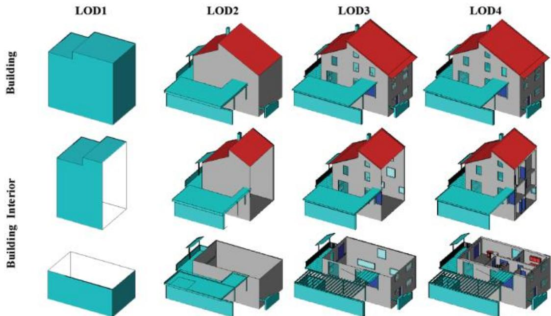
**Figure 19: Illustration of CityGML LOD for buildings (Karlsruhe Institute of Technology)**
