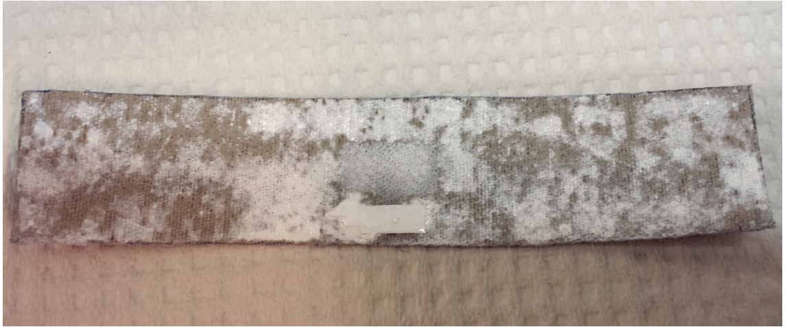
Figure 4.5 Less viscous white glue coated and dried UHF RFID tag.
