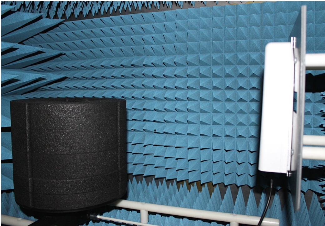
Figure 4.11 Inside view of Voyantic Tagformance Anechoic chamber.
