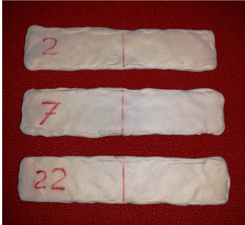
Figure 5.1 Silicon rubber coated tags after 15 washing cycles.
