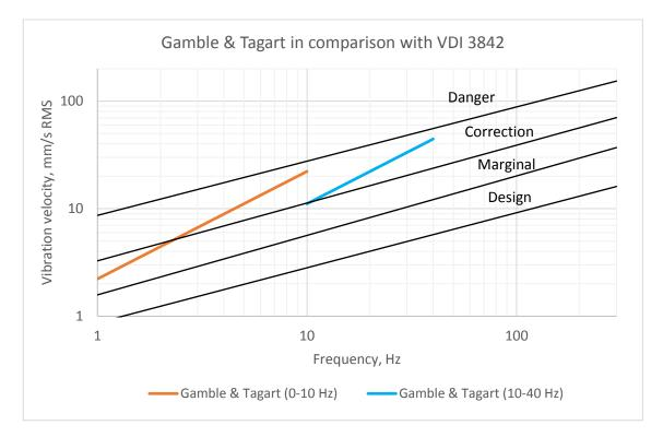
Fig. 61. Vibration velocity limits according to Gamble & Tagart (1991).
