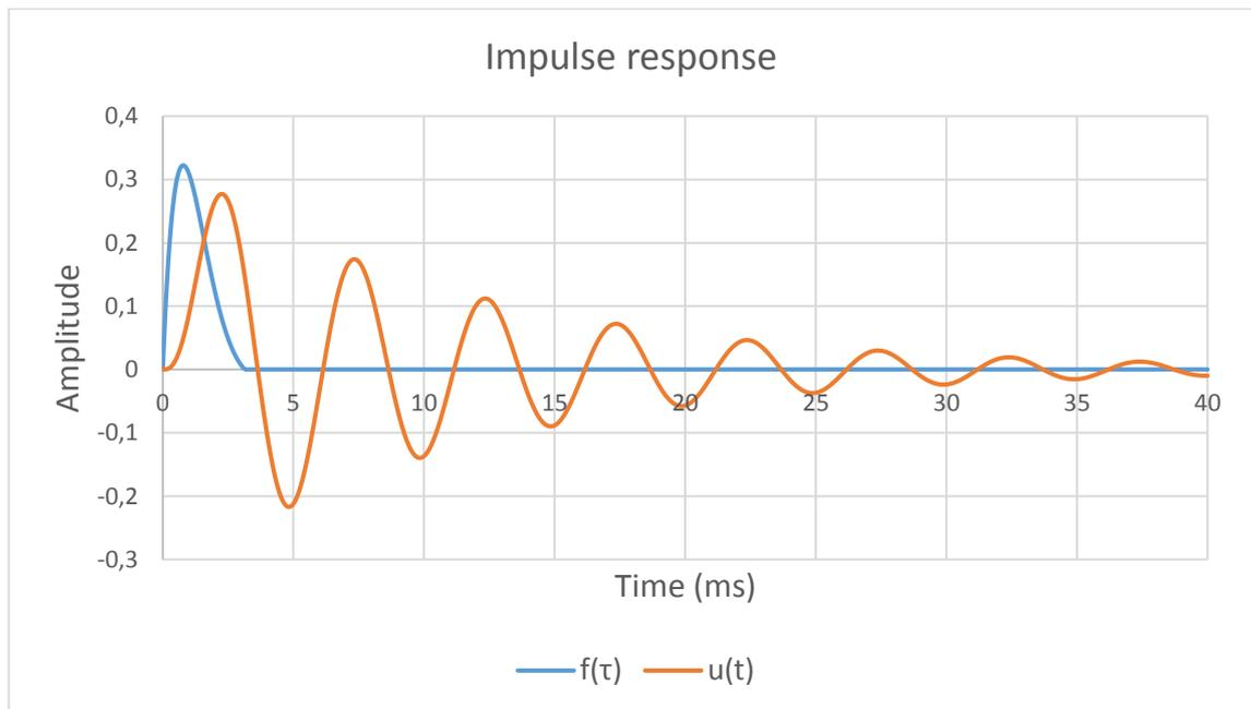
**Fig. 18.** Response of a damped oscillator after an impulse.
