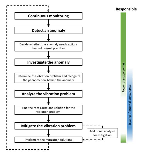
Fig. 20. Workflow for solving pipe vibration problems.
