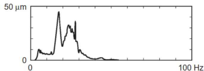
**Fig. 48.** Frequency spectrum of a cavitation vibration problem (Kaneko et al. 2014, p. 247).
