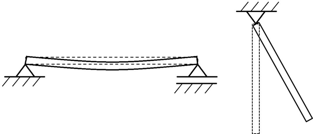
*Fig. 2. A beam and a pendulum deflected from their equilibrium position.*
