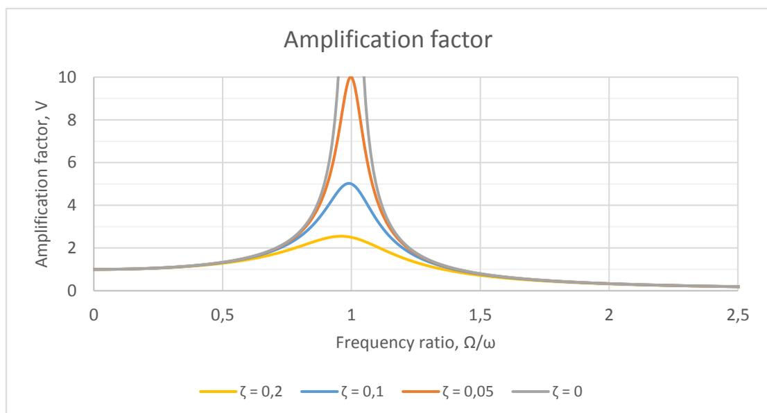
**Fig. 10.** Amplification factor for force-induced vibration.
