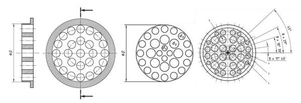
Fig. 31. Different types of flow conditioners: K-Lab (left), NEL (middle), Zanker (right) (ISO 2003).
