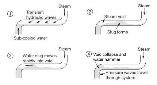
*Fig. 51.* Formation of condensation-induced water hammer (Kaneko et al. 2014, p. 296).
