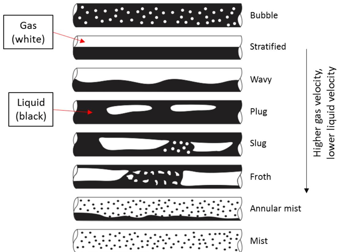
*Fig. 50. Flow patterns in horizontal piping (Kaneko et al. 2014, p. 172).*
