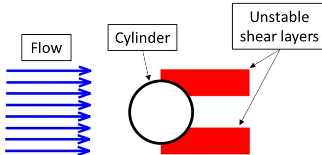
**Fig. 43.** *Unstable shear layers behind the cylinder in outer flow.*
