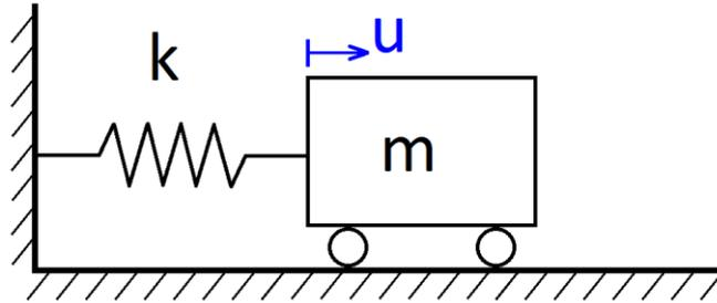
**Fig. 4.** Single degree of freedom mass-spring system.
