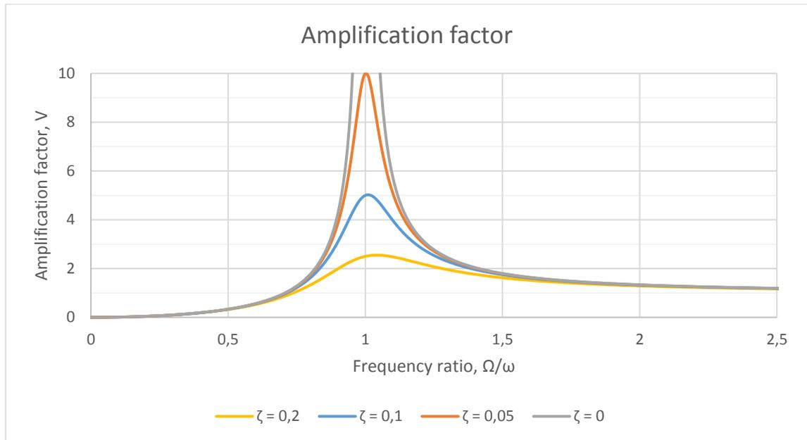
**Fig. 12.** Amplification factor for inertial excitation.
