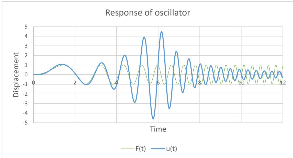
*Fig. 16. Damped oscillator with accelerating excitation frequency.*
