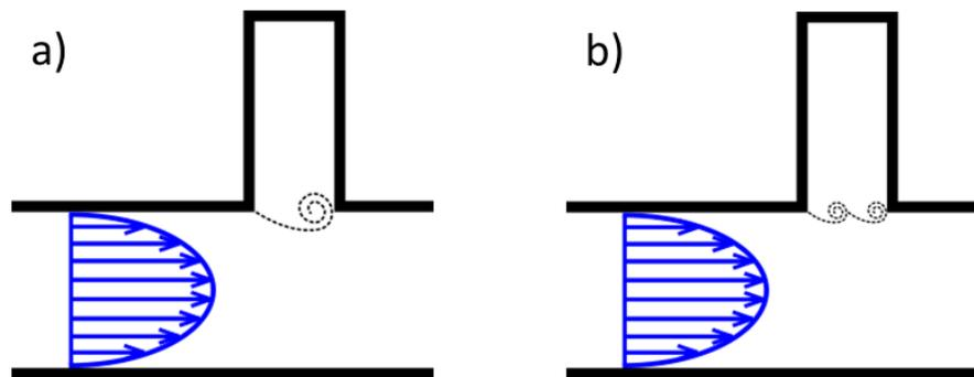
**Fig. 40.** *Vortex shedding in the flow past side branch, a) single vortex mode and b) double vortex mode.*
