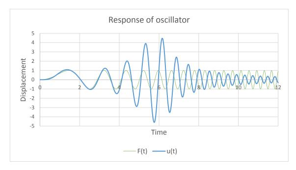
Fig. 16. Damped oscillator with accelerating excitation frequency.
