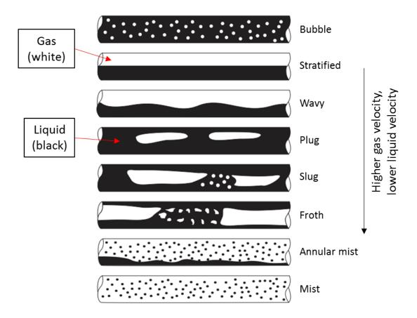
Fig. 50. Flow patterns in horizontal piping (Kaneko et al. 2014, p. 172).
