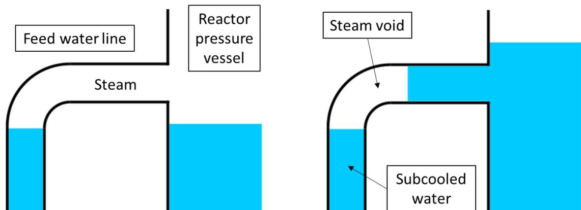
**Fig. 52.** *Condensation-induced water hammer in boiling water reactor feed water line due to rapid water level changes.*
