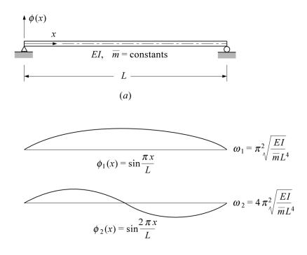
Fig. 5. Two lowest eigenmodes of a simply supported beam and their analytical solutions (Clough & Penzien 2003, p. 380).
