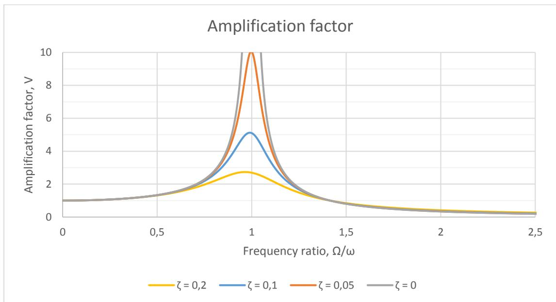
*Fig. 14. Amplification factor for foundation-induced excitation.*
