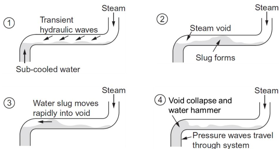
**Fig. 51.** Formation of condensation-induced water hammer (Kaneko et al. 2014, p. 296).
