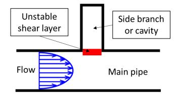
Fig. 39. Unstable shear layer in piping.
