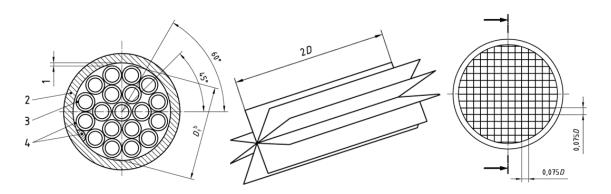
Fig. 30. Different types of flow straighteners: tube bundle (left), Étoile straightener (middle), AMCA straightener (right) (ISO 2003).
