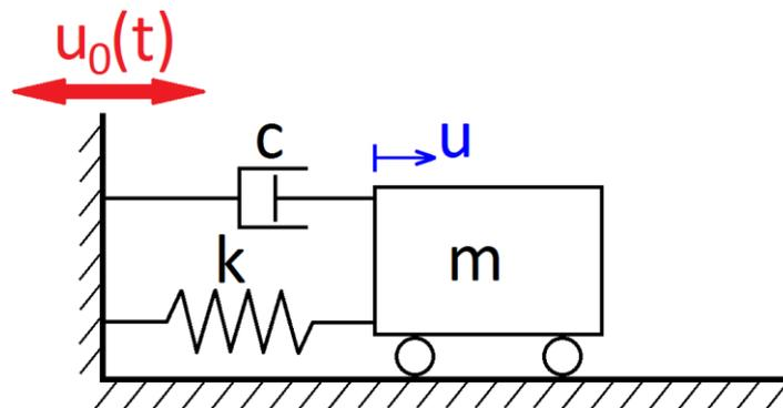
**Fig. 13.** Vibratory displacement of foundation.
