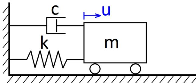
**Fig. 6.** Damped mass-spring system.
