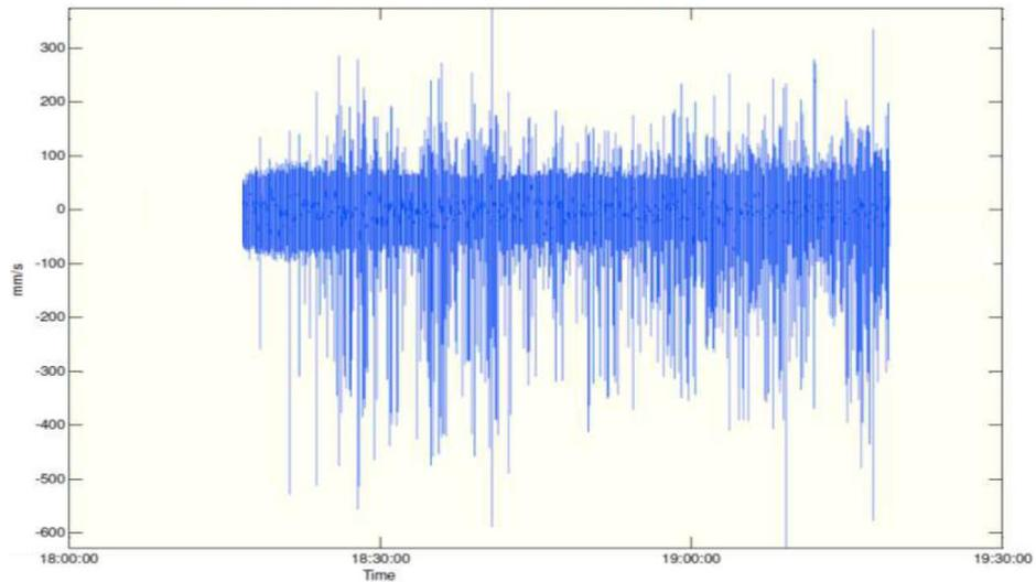
*Fig. 56. Example of random vibrations response in time domain.*
