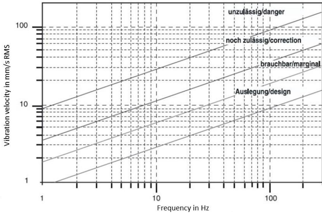
*Fig. 60. Vibration velocity limits according to VDI 3842:2004-6.*
