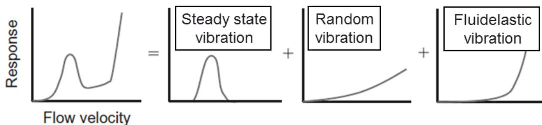
**Fig. 37.** Types of flow-induced vibrations (Kaneko et al. 2014, p. 9).
