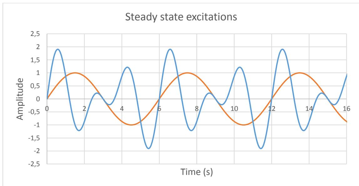
*Fig. 15. Two steady state excitations: the orange is pure sine wave and the blue is two summed sine waves.*
