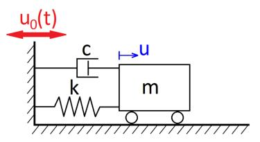
Fig. 13. Vibratory displacement of foundation.
