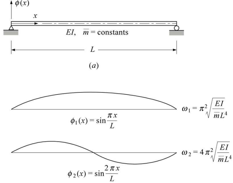
**Fig. 5.** Two lowest eigenmodes of a simply supported beam and their analytical solutions (Clough & Penzien 2003, p. 380).
