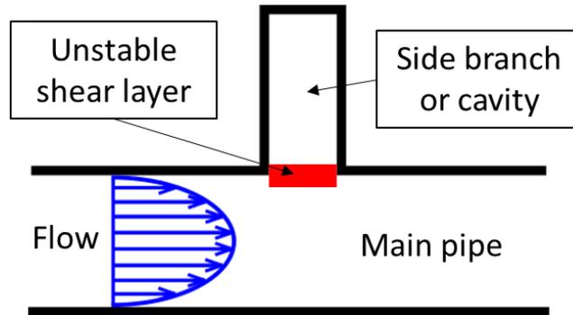
**Fig. 39.** *Unstable shear layer in piping.*
