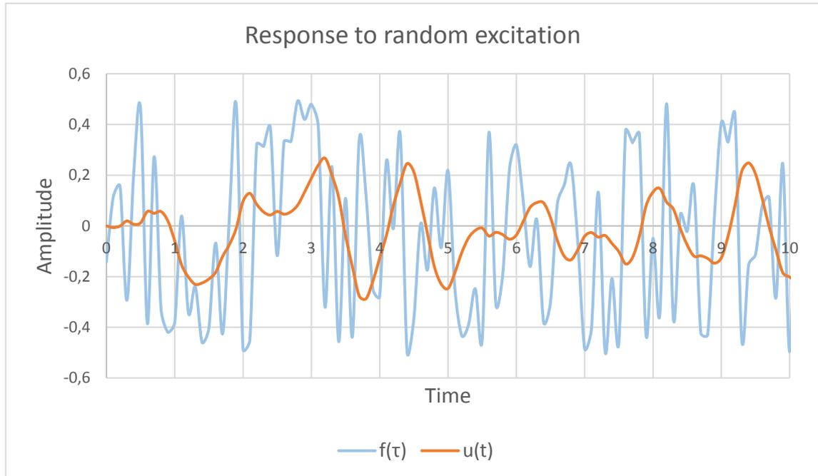
**Fig. 19.** An example of system response to random force-induced excitation.
