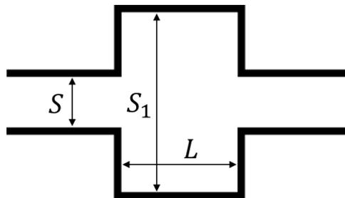
*Fig. 35. Acoustic damper / Surge drum.*
