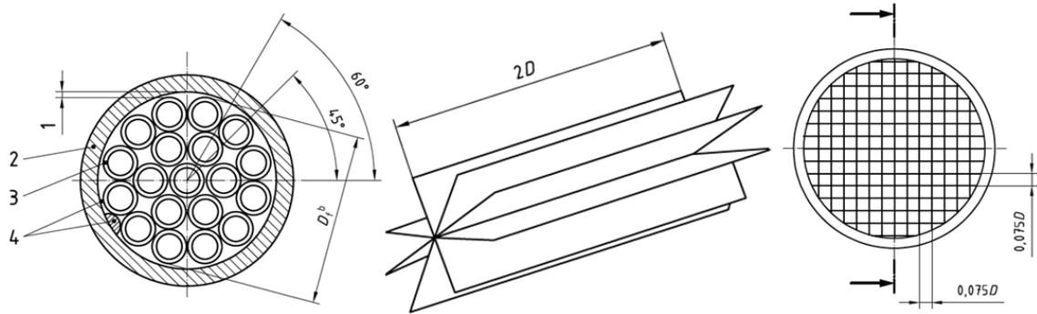
**Fig. 30.** Different types of flow straighteners: tube bundle (left), Étoile straightener (middle), AMCA straightener (right) (ISO 2003).
