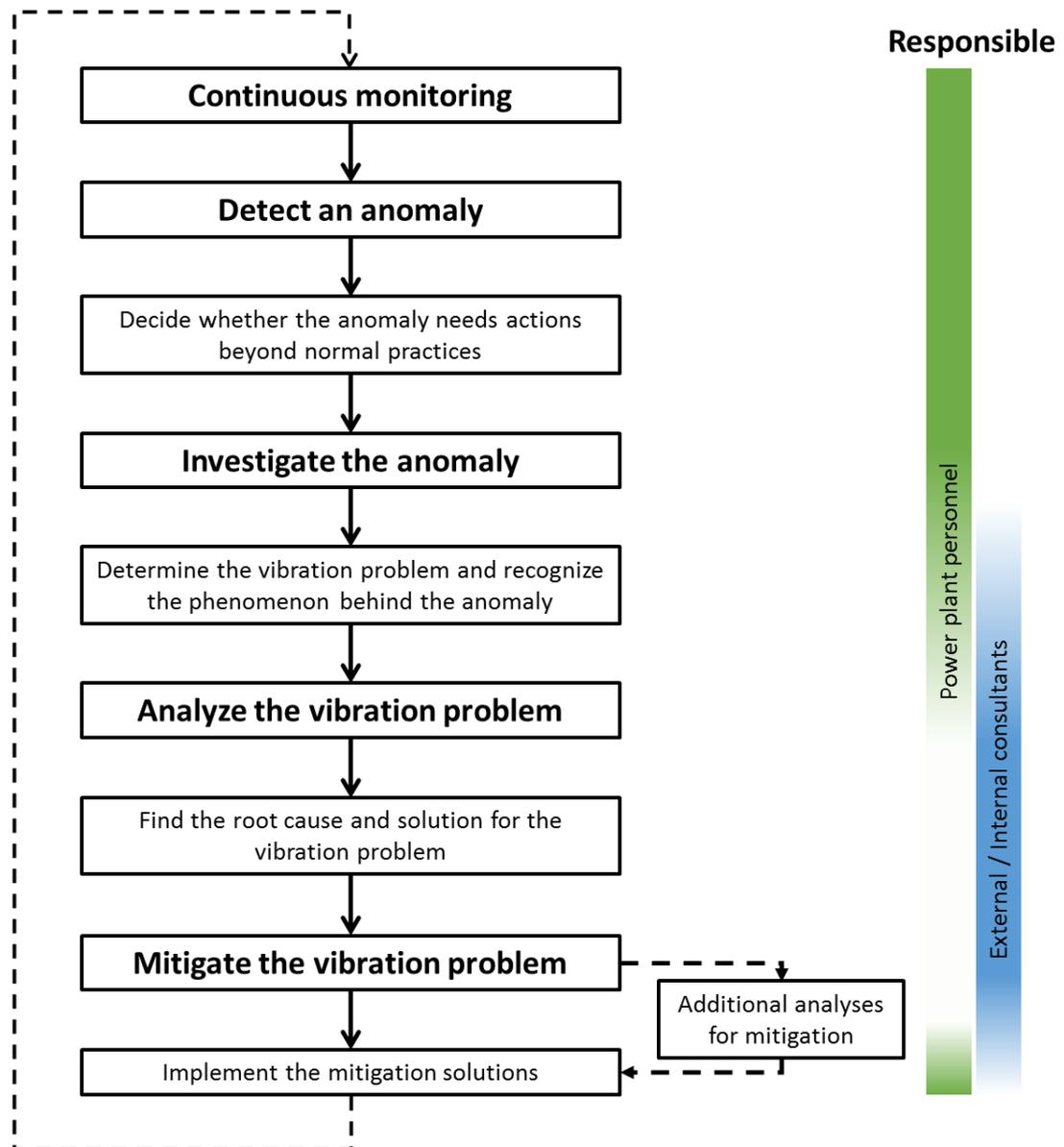
*Fig. 20. Workflow for solving pipe vibration problems.*
