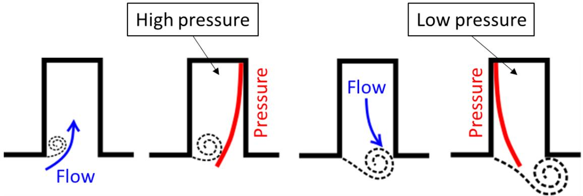
**Fig. 41.** Vortex shedding in combination with side branch acoustic resonance (Dequand et al. 2003).
