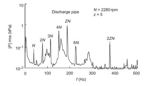
Fig. 46. Frequency spectrum of pressure pulsations created by a centrifugal pump, Z = number of impeller blades (Kaneko et al. 2014, p. 222).
