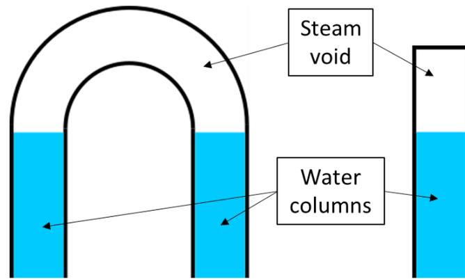
**Fig. 53.** *Column separation in high point and closed end.*
