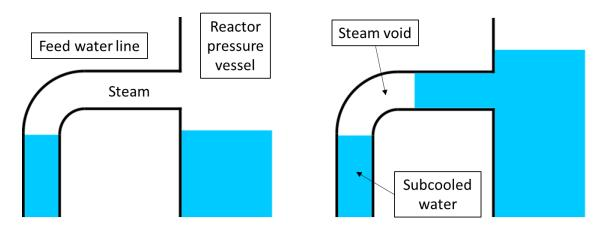
*Fig. 52.* Condensation-induced water hammer in boiling water reactor feed water line due to rapid water level changes.
