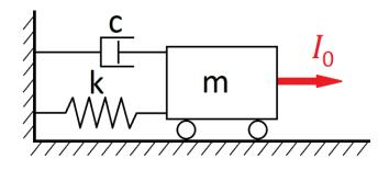
Fig. 17. Impulse applied to the body.
