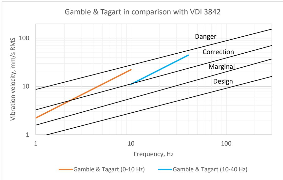
**Fig. 61.** *Vibration velocity limits according to Gamble & Tagart (1991).*
