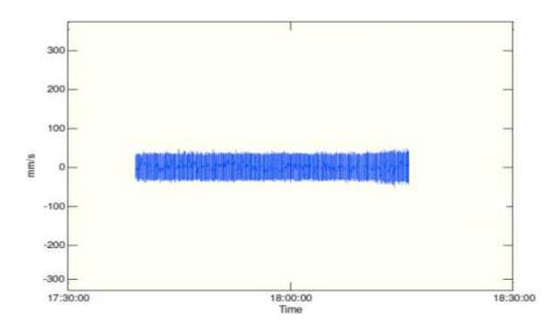
Fig. 54. Example of steady state vibrations response in time domain.
