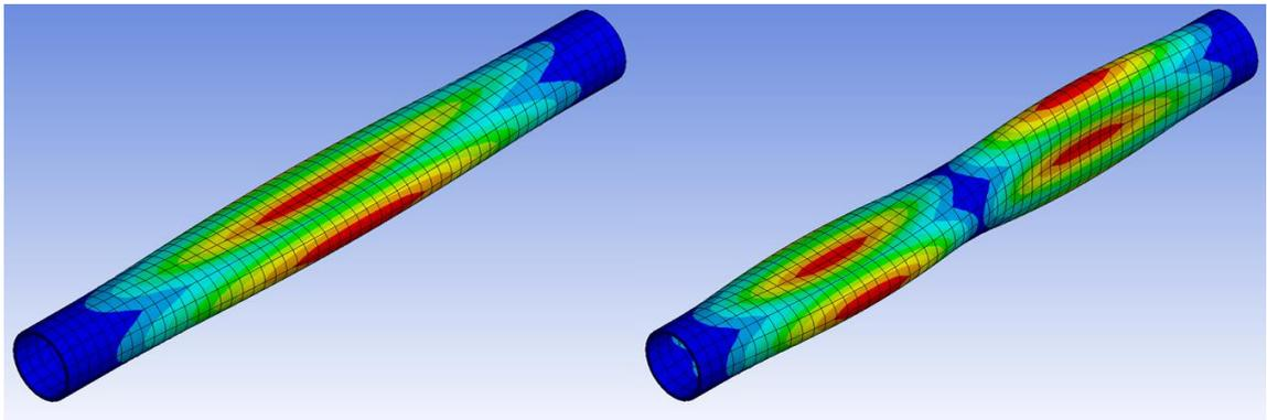
*Fig. 3. The two lowest pipe wall natural modes.*
