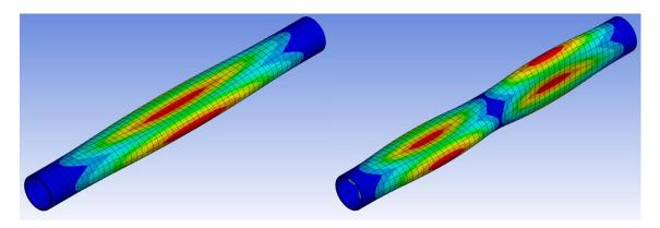
Fig. 3. The two lowest pipe wall natural modes.
