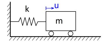
Fig. 4. Single degree of freedom mass-spring system.
