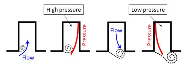
*Fig. 41.* Vortex shedding in combination with side branch acoustic resonance (Dequand et al. 2003).
