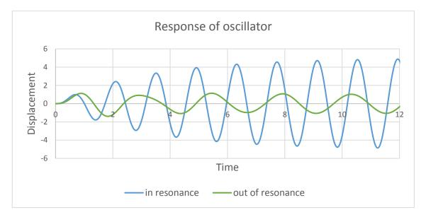
Fig. 8. Damped oscillator in resonance and out of resonance.
