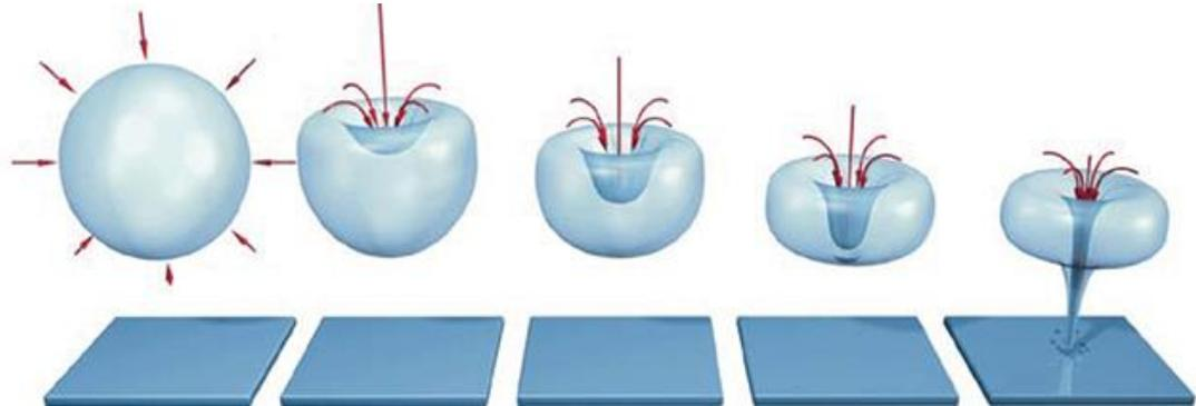
**Fig. 47.** Vapor bubble collapse in cavitation (MCOR 2017).
