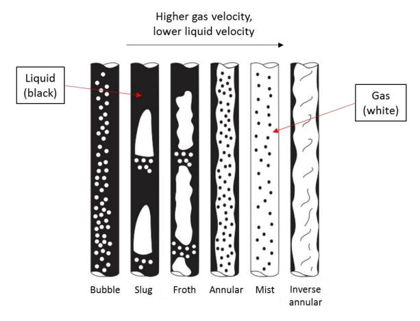
Fig. 49. Flow patterns in vertical piping (Kaneko et al. 2014, p. 171).
