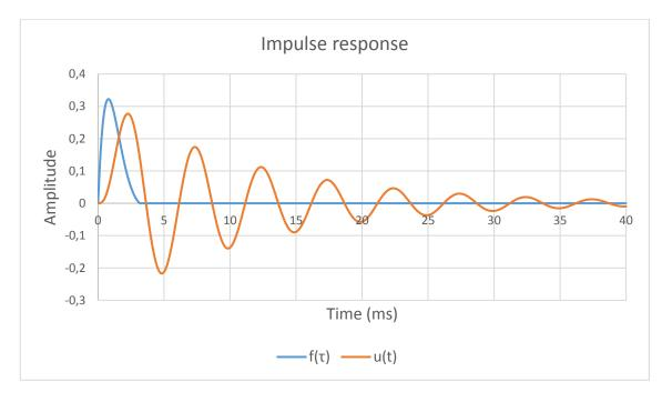
Fig. 18. Response of a damped oscillator after an impulse.
