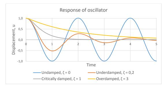
Fig. 7. The responses of oscillator with different damping ratios.
