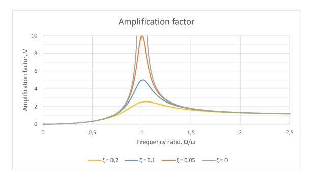
Fig. 12. Amplification factor for inertial excitation.
