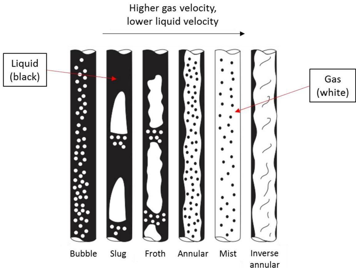
**Fig. 49.** Flow patterns in vertical piping (Kaneko et al. 2014, p. 171).
