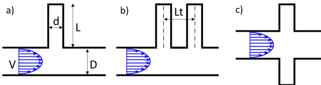
**Fig. 42.** Side branch configurations a) single, b) tandem and c) coaxial.
