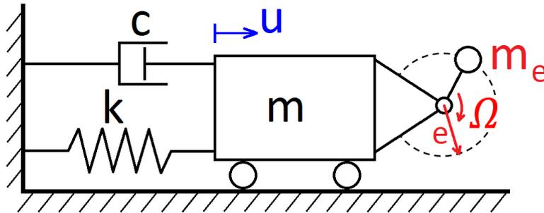
**Fig. 11.** Force generated within the rigid body.
