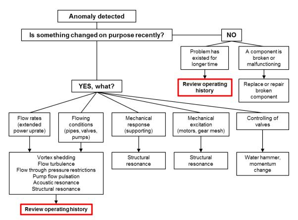
Fig. 27. Flow chart for checking the recent changes.
