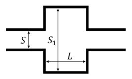
Fig. 35. Acoustic damper / Surge drum.
