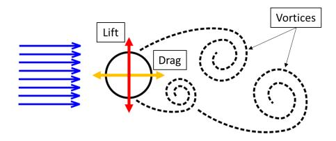
Fig. 44. Vortices behind the cylinder in outer flow.
