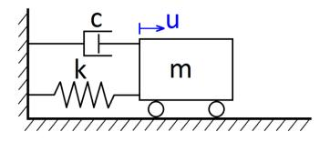
Fig. 6. Damped mass-spring system.
