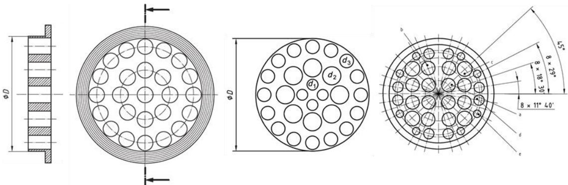
**Fig. 31.** Different types of flow conditioners: K-Lab (left), NEL (middle), Zanker (right) (ISO 2003).
