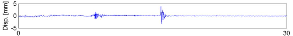
*Fig. 58. Example of rapid transient vibrations response in time domain.*
