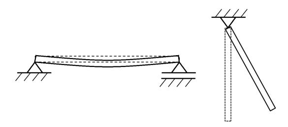
Fig. 2. A beam and a pendulum deflected from their equilibrium position.
