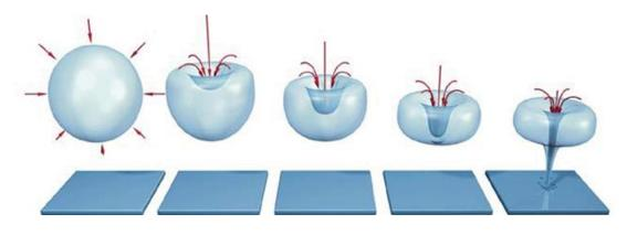
Fig. 47. Vapor bubble collapse in cavitation (MCOR 2017).
