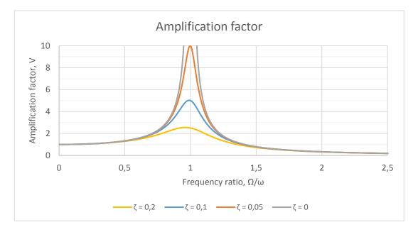
Fig. 10. Amplification factor for force-induced vibration.
