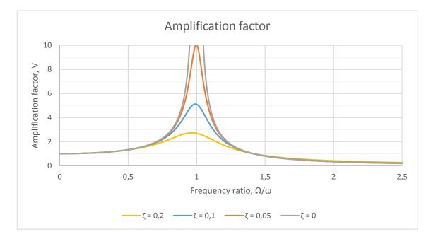
Fig. 14. Amplification factor for foundation-induced excitation.
