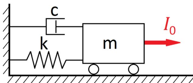
*Fig. 17. Impulse applied to the body.*
