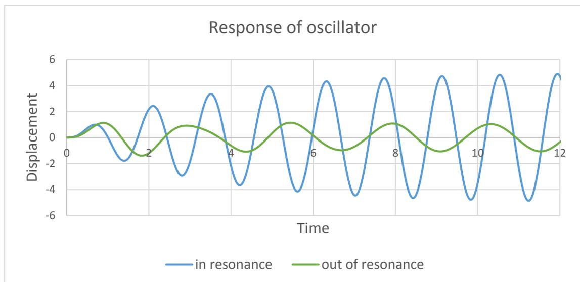
**Fig. 8.** Damped oscillator in resonance and out of resonance.
