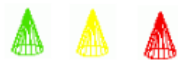
Figure 2.6. Connection and detail components' color symbols the component creation status. (Green-successfully, Yellow-created but has problems, and Red-not created)
