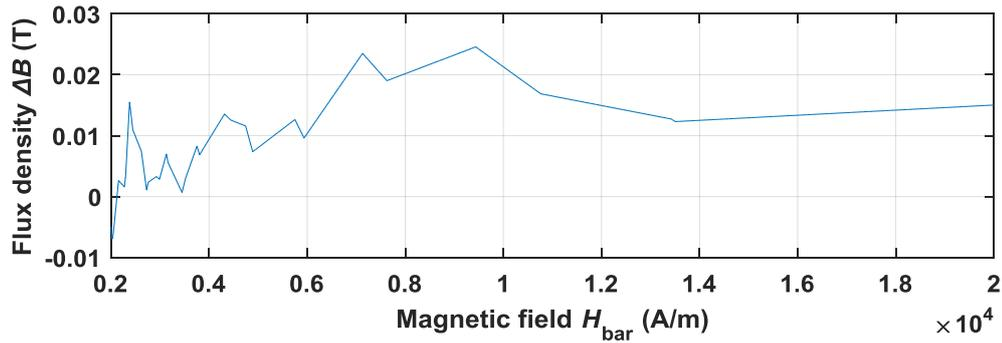
**Figure 6.4b:**  $\Delta B$  for zero to 20 MPa compressive stress.
