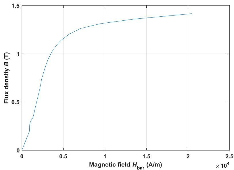
*Figure 6.2: Single valued  $B$ - $H$  curve for the stack of steel sheets.*
