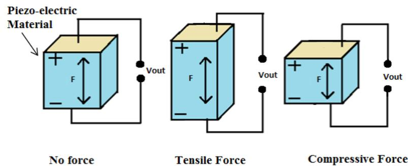
*Figure 2.6: Working principle of piezo-electric transducer.*
