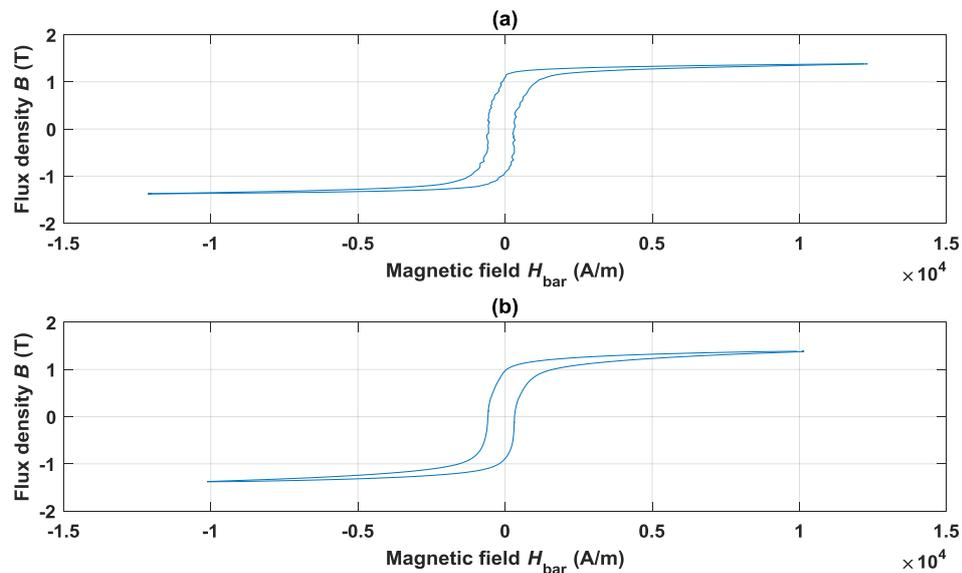
**Figure 7.1:**  $B$ - $H$  curve before filtration (a) and after filtration (b) of the measured voltage and magnetizing current.
