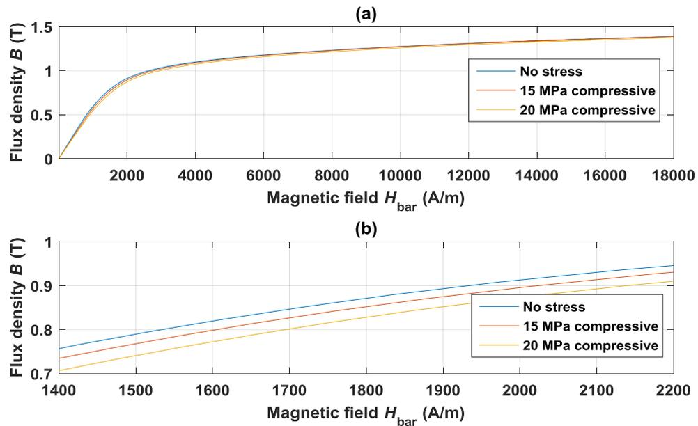
**Figure 6.7:** Weighted averaged B-H curves (a) and the scaled plot (b) under compressive stress.
