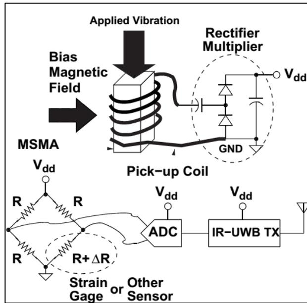
**Figure 2.22:** Test setup for energy harvesting using MSMA material and wireless sensor system [39].
