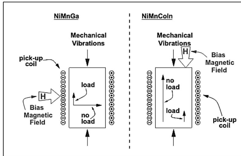
*Figure 2.23: Different methods of magnetic field biasing on test samples under mechanical loading [39].*
