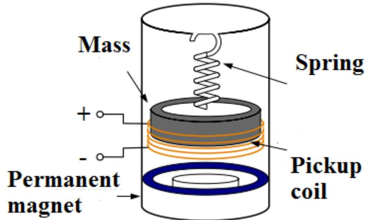
*Figure 2.4: Working principle of an electromagnetic energy harvester [23].*
