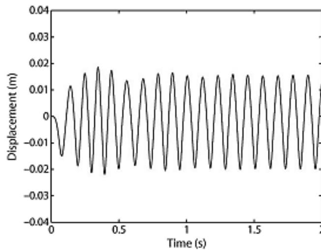
**Figure 2.15:** Central magnet's relative displacement under harmonic based excitation [7].
