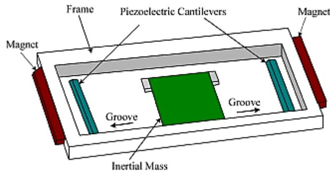
*Figure 2.21: Impact coupling type PZT based energy harvesting device [4].*
