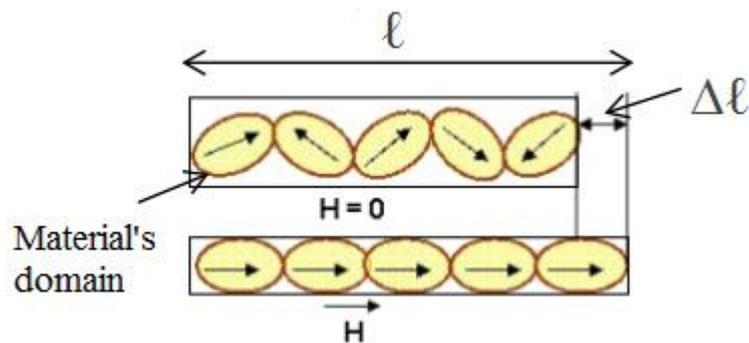
**Figure 2.2:** *Magnetostriction and domain walls rearrangement in ferromagnetic materials under applied magnetic field.*
