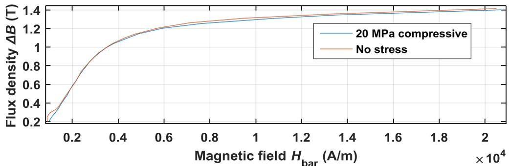
**Figure 6.4a:**  $B$ - $H$  curves for zero and 20 MPa compressive stress.
