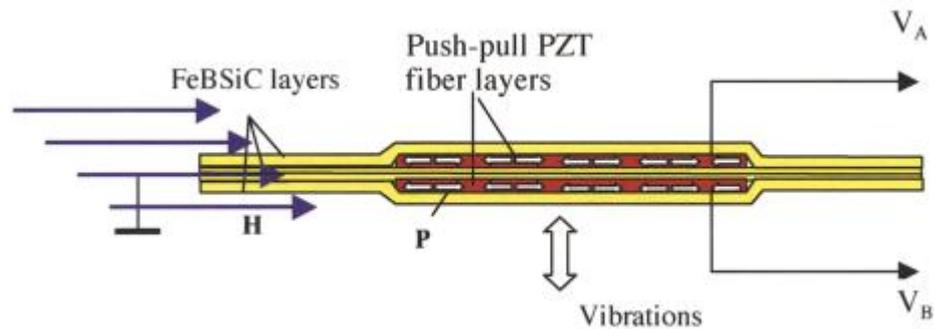
**Figure 2.17:** Magneto electric energy harvesting device [34].
