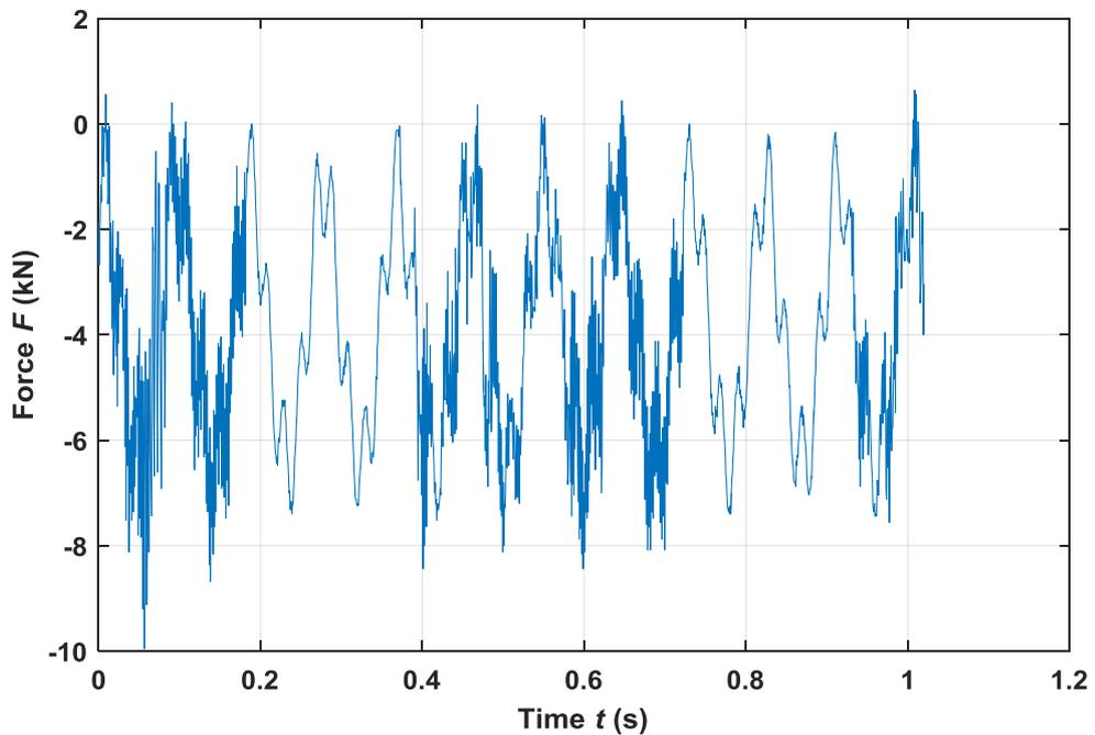
**Figure 7.5:** *Cyclic loading at 11 Hz from 0 kN to -8 kN.*
