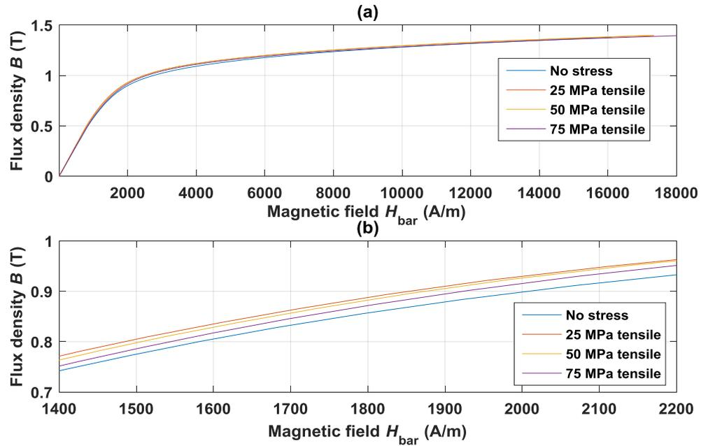
**Figure 6.6:** Weighted averaged B-H curves (a) and the scaled plot (b) under different tensile stress values.
