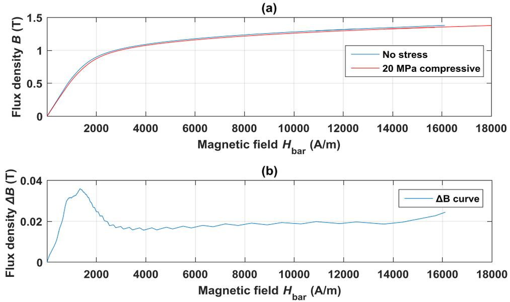
**Figure 6.9:** The weighted averaged  $B$ - $H$  curves (a) and the  $\Delta B$  curve (b) for 0 and 20 MPa compressive stress.
