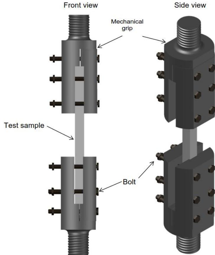
*Figure 4.3:* 3D model of mechanical grips holding the test sample.
