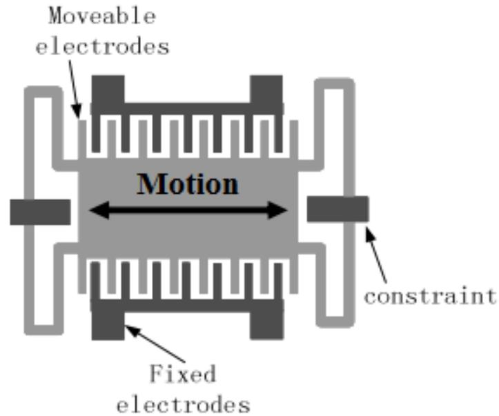
**Figure 2.3:** *Electrostatic energy harvesting using variable capacitor under horizontal vibration [20].*
