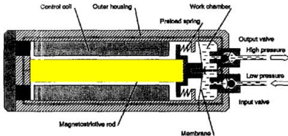
*Figure 3.3: Magnetostrictive material based high pressure fluid pump [24].*
