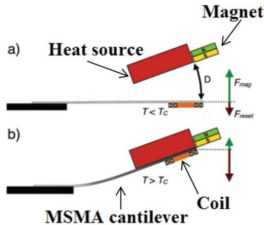
**Figure 2.12:** Principle of operation in MSMA based energy harvesting device in [9].
