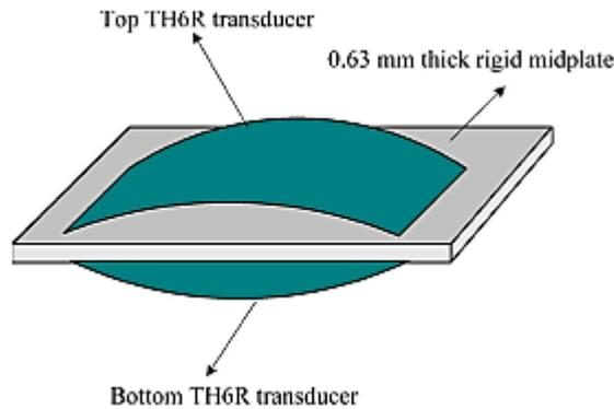
*Figure 2.20: Piezoelectric based bimorph transducer [4].*
