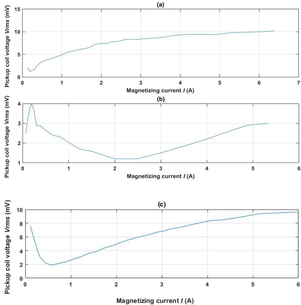
**Figure 6.10:** Pickup coil voltage and magnetizing current for (a) 2.5 MPa to 25MPa, (b) zero to -20 MPa and (c) 15 MPa to -15 MPa using stack of steel sheets sample.
