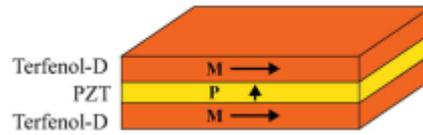
**Figure 2.14:** Magneto-electric laminate composed of PZT layer sandwiched between layers of Terfenol-D [7].
