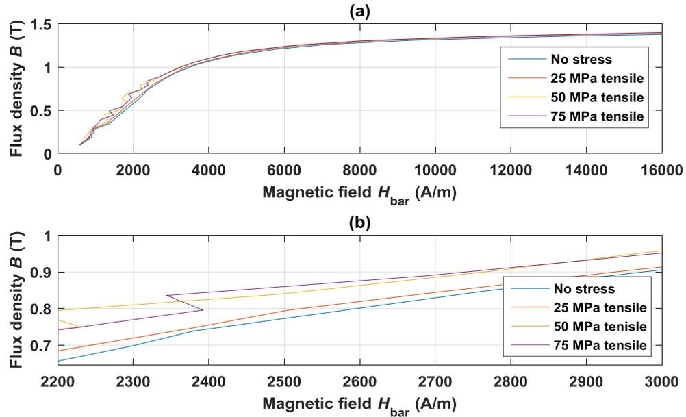
**Figure 6.3:**  $B$ - $H$  curves under different tensile stress values (a) and the scaled plot (b) showing the effect of mechanical stress.
