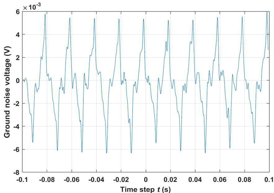
**Figure 7.6:** Measured ground noise voltage.
