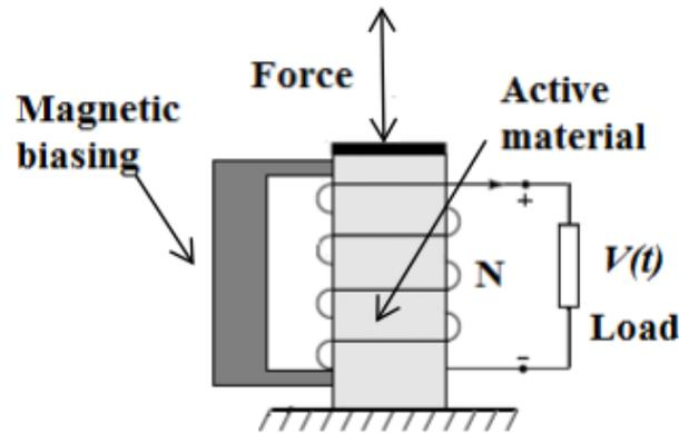
**Figure 2.7:** Schematic of magnetostrictive material based energy harvesting device.
