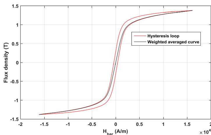
**Figure 6.5:** Hysteresis loop and weighted average curve without mechanical stress.
