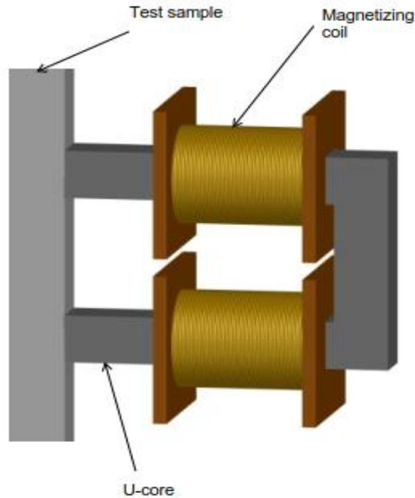
**Figure 4.4:** 3D model of the magnetizing coil and U-core.
