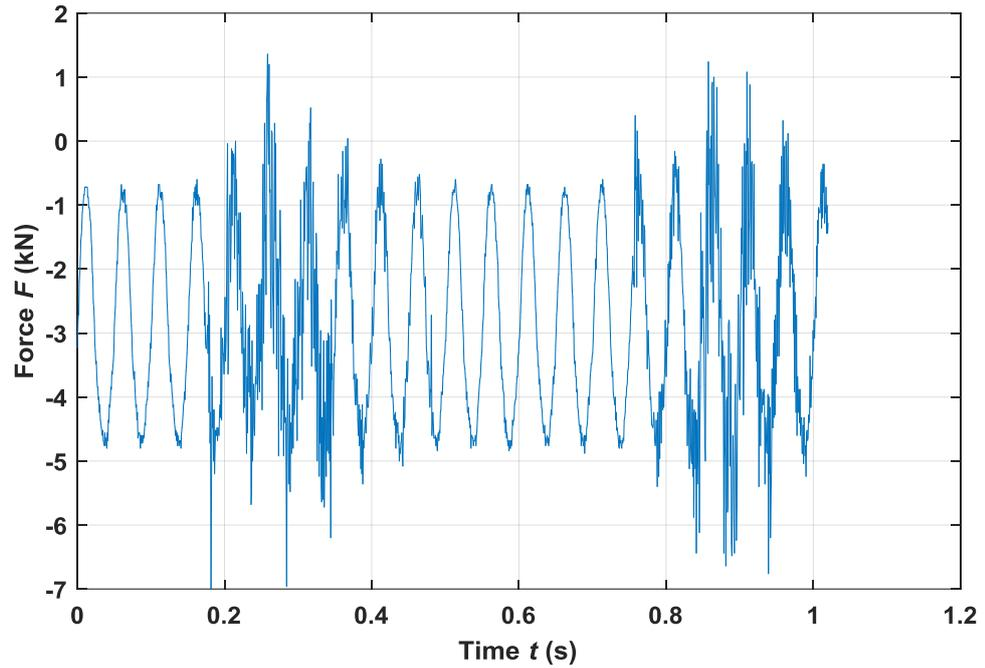
**Figure 7.4:** *Cyclic loading at 20 Hz from -1kN to -5 kN.*
