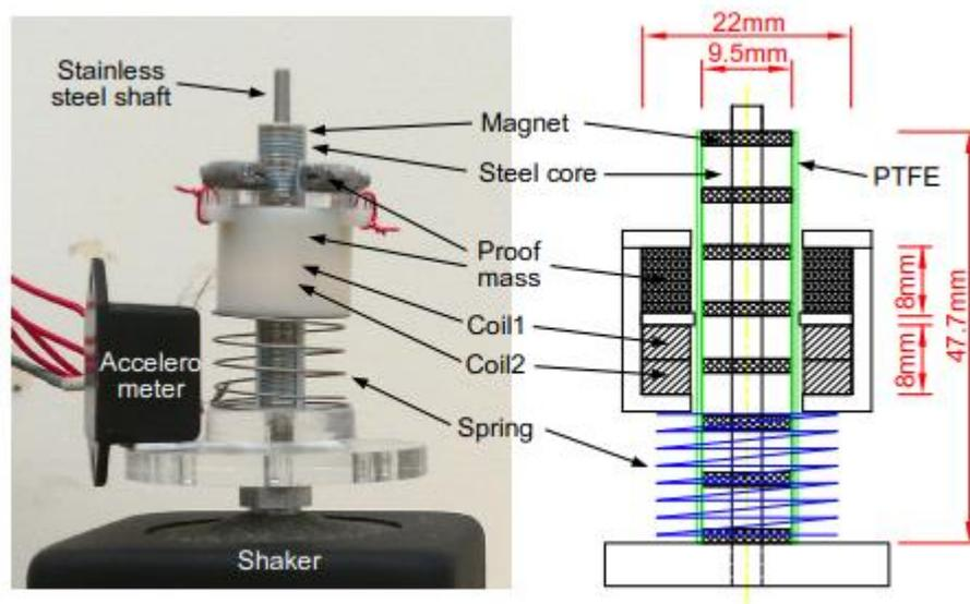
**Figure 2.11:** Prototype device for electromagnetic energy harvester [31].
