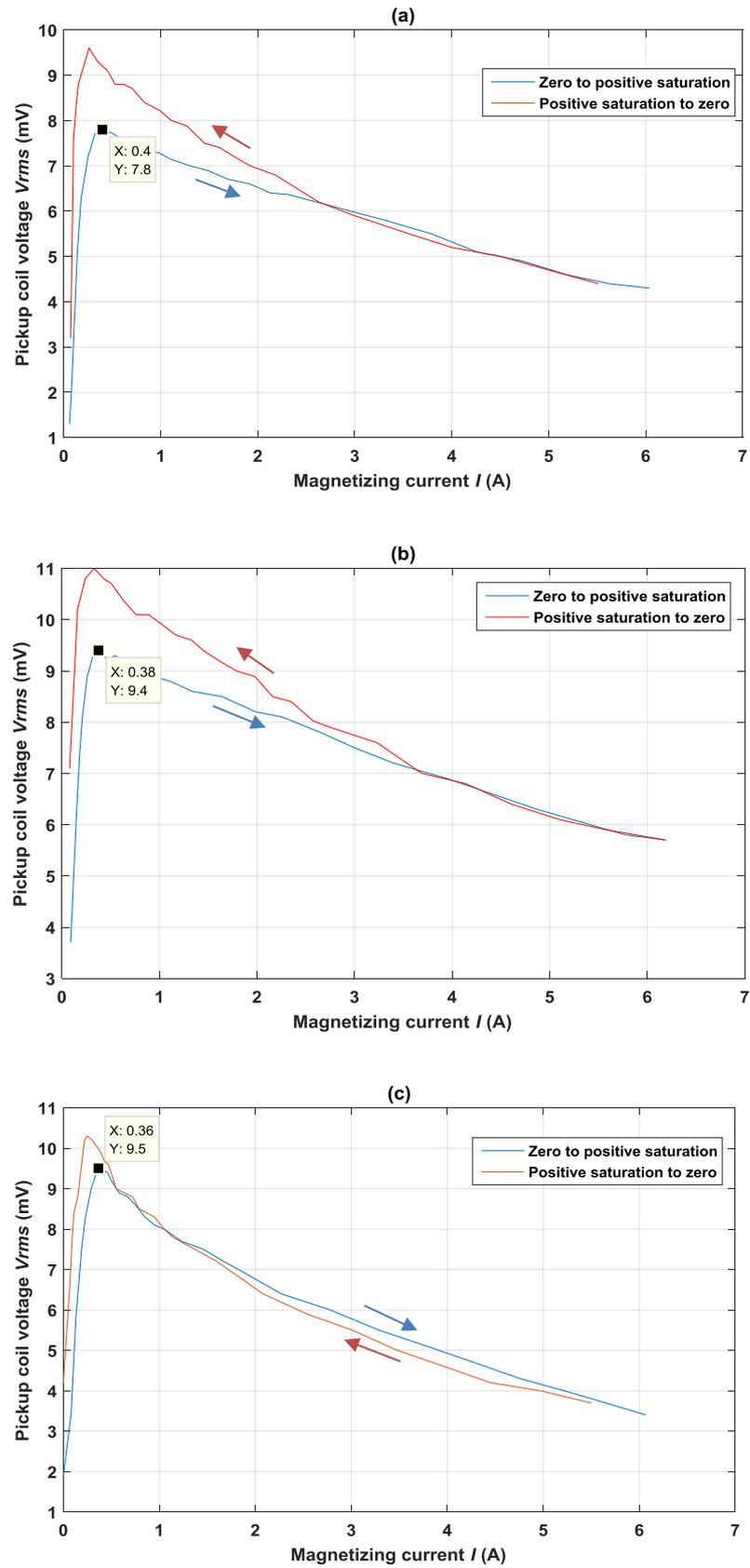
**Figure 6.11:** Plot for induced voltage and magnetizing current for (a) 2.5 MPa to 25MPa, (b) 15 MPa to -15 MPa and (c) 0 MPa to -20 MPa using solid test sample.
