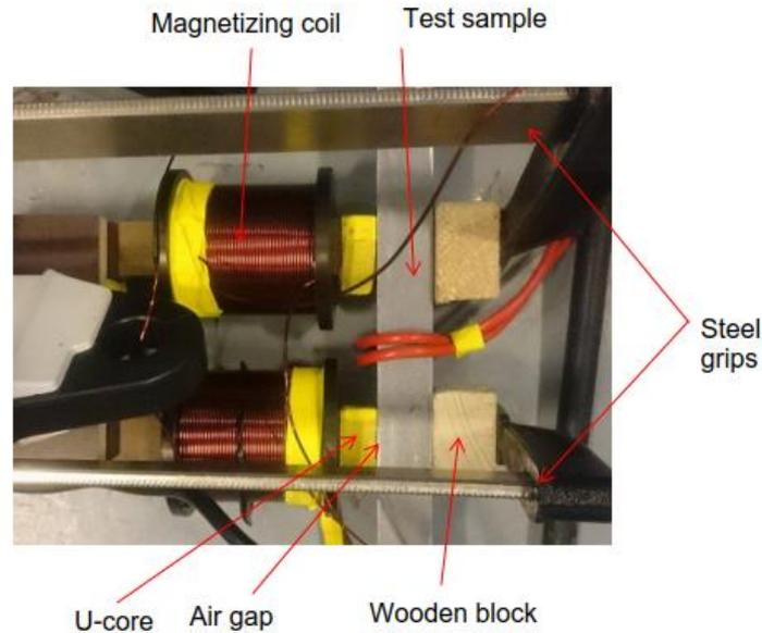
**Figure 7.3:** Steel grips holding the test sample and the magnetizing coil.
