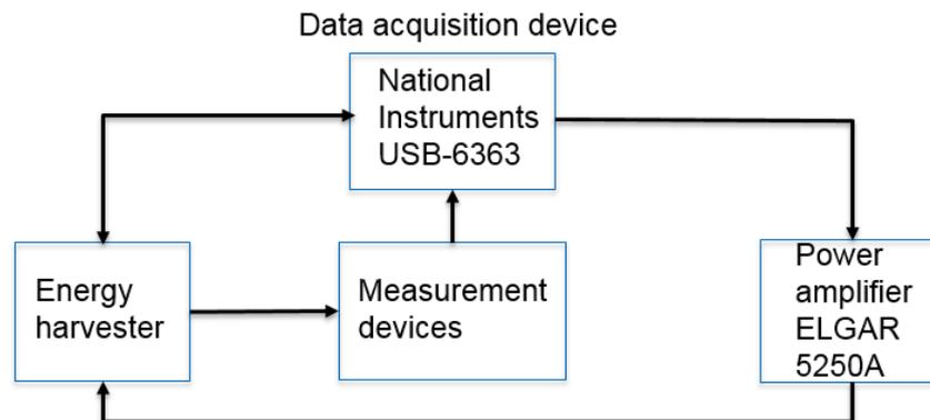
**Figure 4.8:** Block diagram explaining the steps involved to measure magnetization curves.
