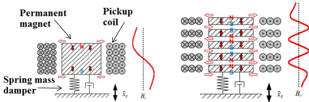
**Figure 2.9:** Single layer electromagnet energy harvester.
