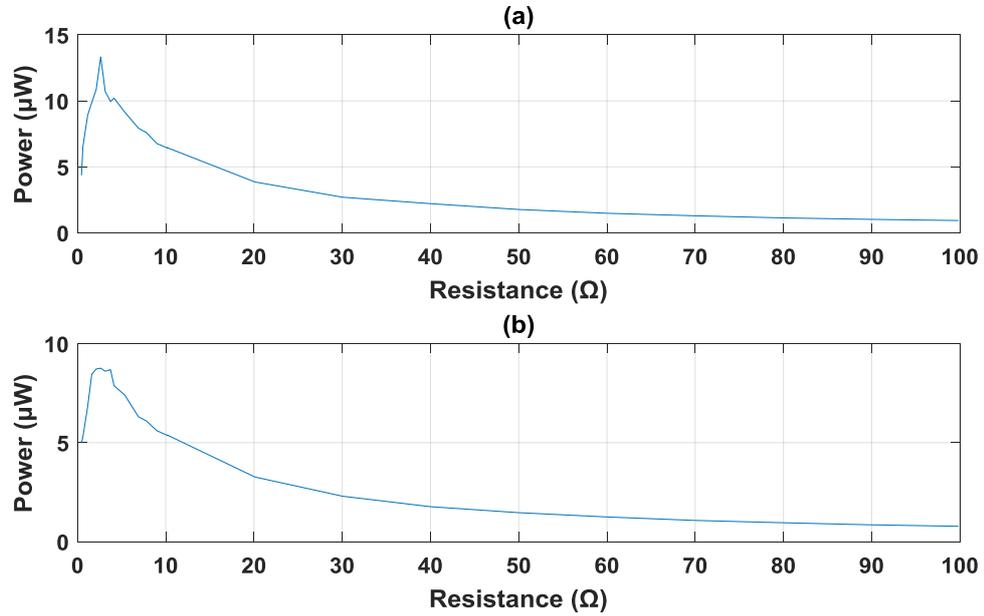
**Figure 6.12:** Output power for zero to -20 MPa (a) and 2.5MPa to 25 MPa (b) of cyclic stress values
