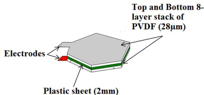
*Figure 2.19: Polyvinylidene fluoride based energy harvesting laminate [4].*
