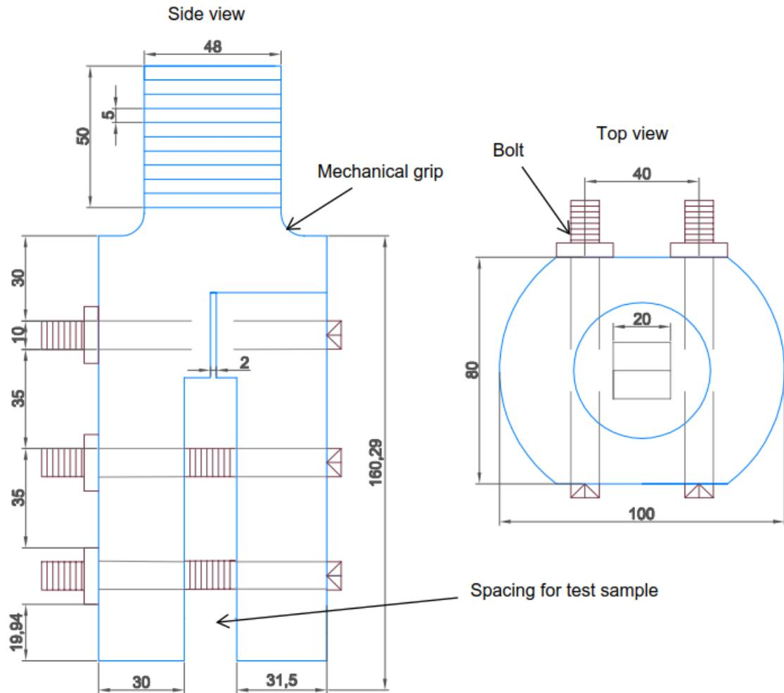
**Figure 4.2:** Schematic diagram of the mechanical grip including overall dimensions.
