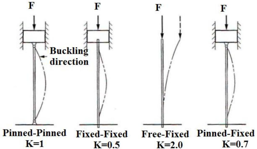
*Figure 4.1: Buckling for different end support conditions [57].*
