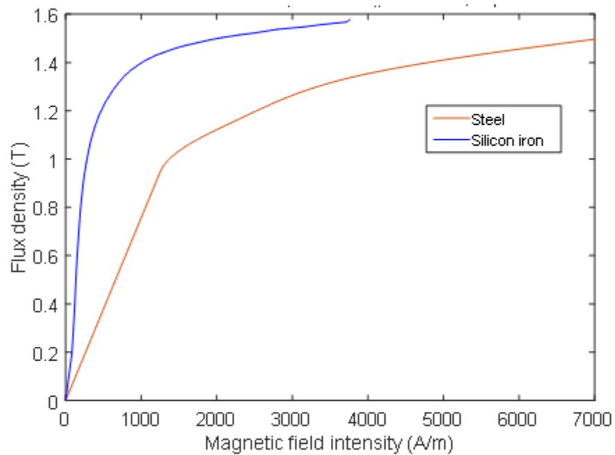
**Figure 4.5:** B-H curves for steel bar and core.
