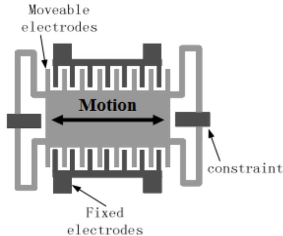
*Figure 2.8: Schematic diagram of electrostatic energy harvester (in-plane gap structure) [30].*
