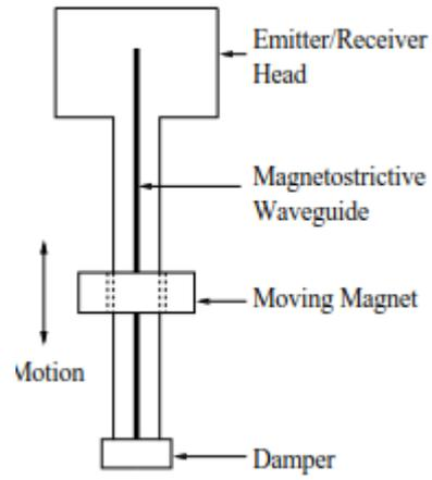
*Figure 3.4: position sensor based on magnetostrictive waveguide [11].*
