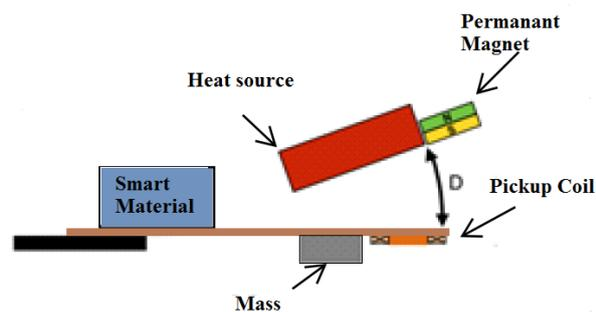
*Figure 2.5: Cantilever based design of thermal energy harvester.*
