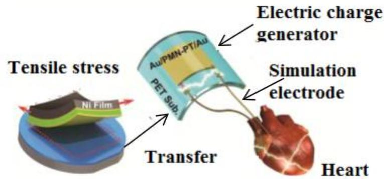
*Figure 3.1: Piezo-electric based pacemaker device [44].*
