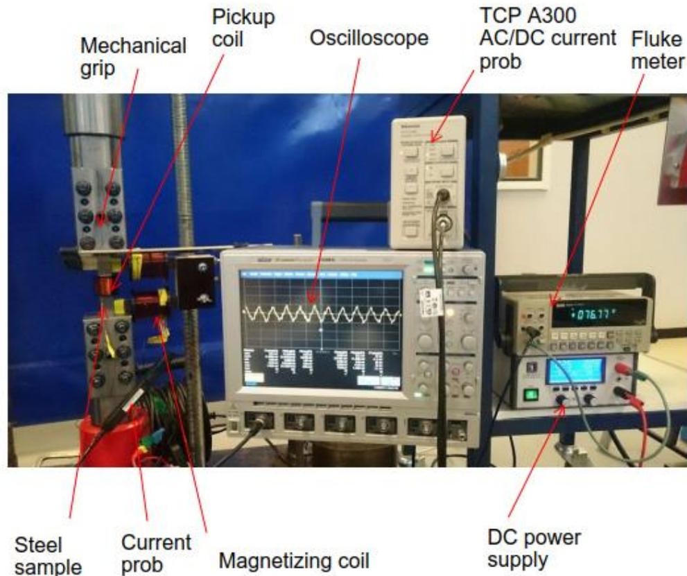
**Figure 4.9:** Experimental setup of the energy harvester.
