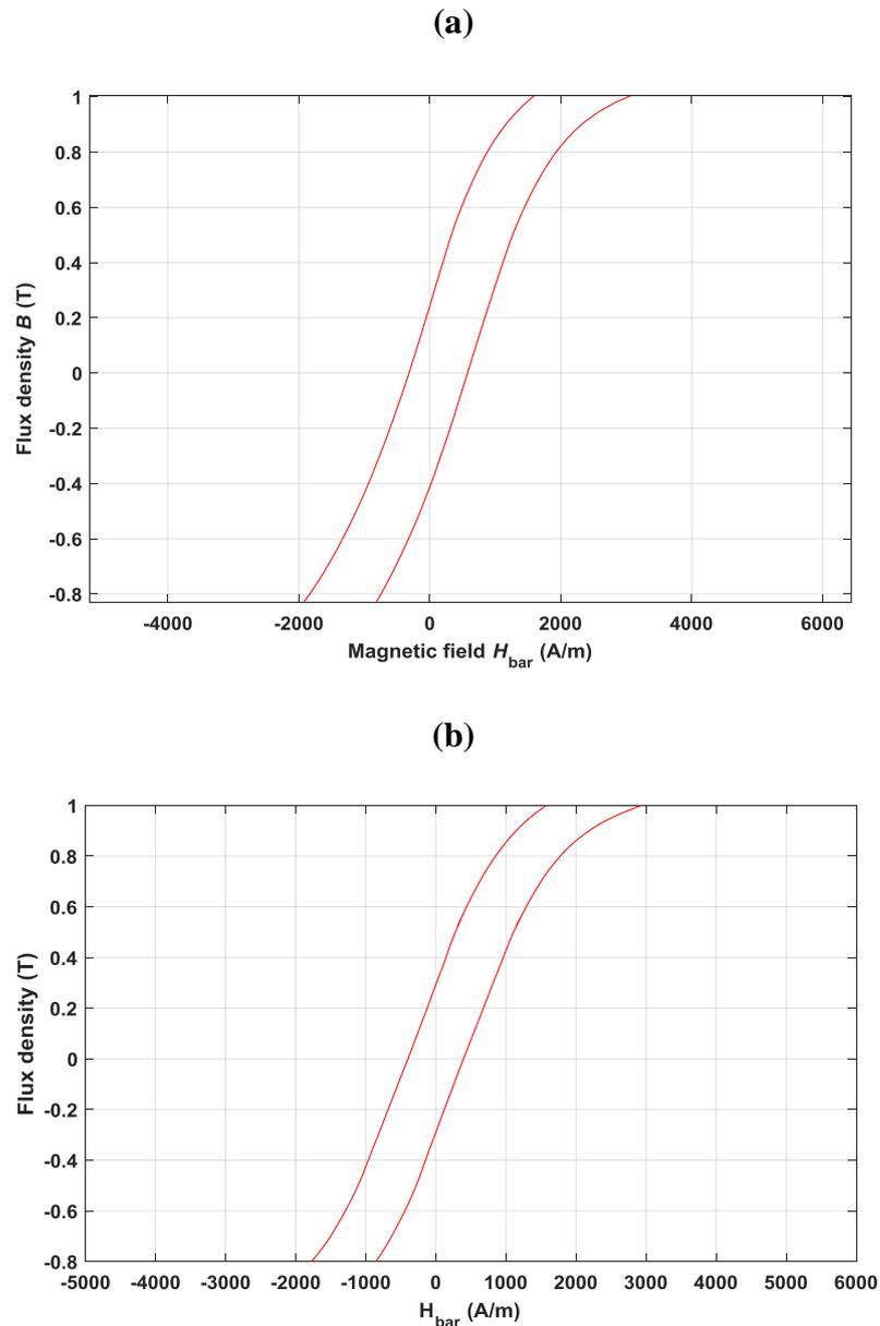
**Figure 7.2:** Scaled plot showing shifting of  $B$ - $H$  hysteresis loop from the origin (a) and the hysteresis loop centered in the origin (b).
