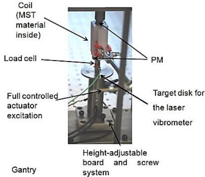
*Figure 2.24: Experimental setup of magnetostrictive energy harvester [40].*
