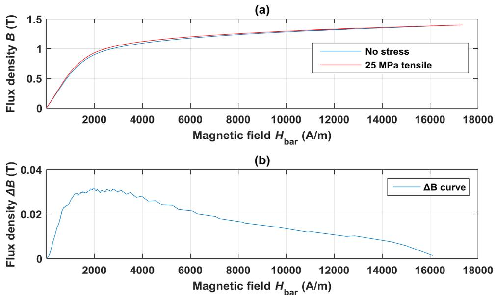
**Figure 6.8:** The weighted averaged  $B$ - $H$  curves (a) and the  $\Delta B$  curve (b) for 0 and 25 MPa tensile stress.
