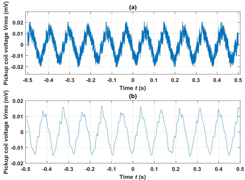
**Figure 7.7:** Output voltage without filtration (a) and the output voltage after using low pass filter (b).
