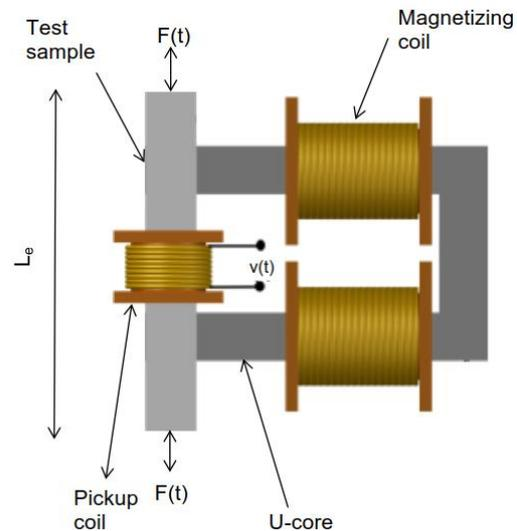
**Figure 4.7b:** Magnetic circuit for energy harvester.
