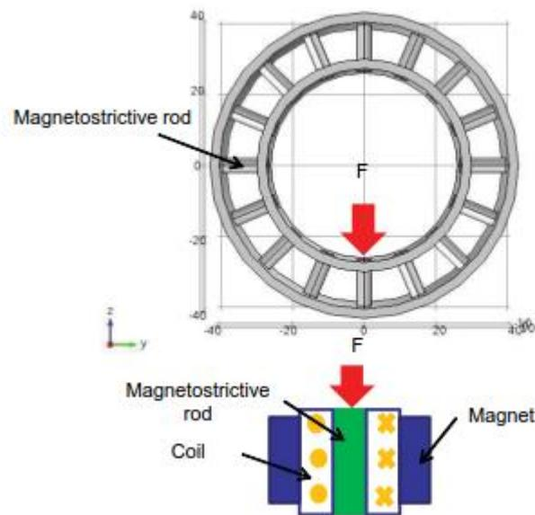
*Figure 3.2: Vibration ring and energy harvesting device setup [53].*
