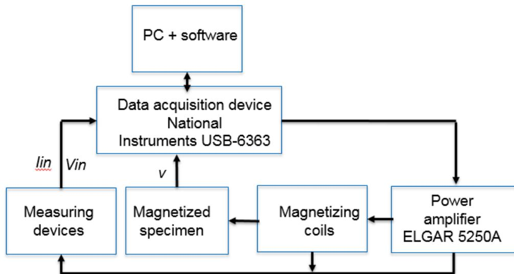
*Figure 5.1: Block diagram of the experimental setup for measuring magnetization curves.*
