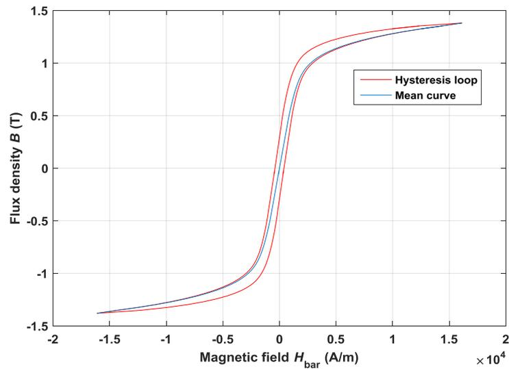
**Figure 5.3:** Hysteresis loop and weighted averaged  $B$ - $H$  curve of the test sample.
