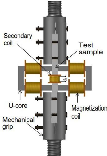
**Figure 4.7a:** Working principle of the energy harvesting device.
