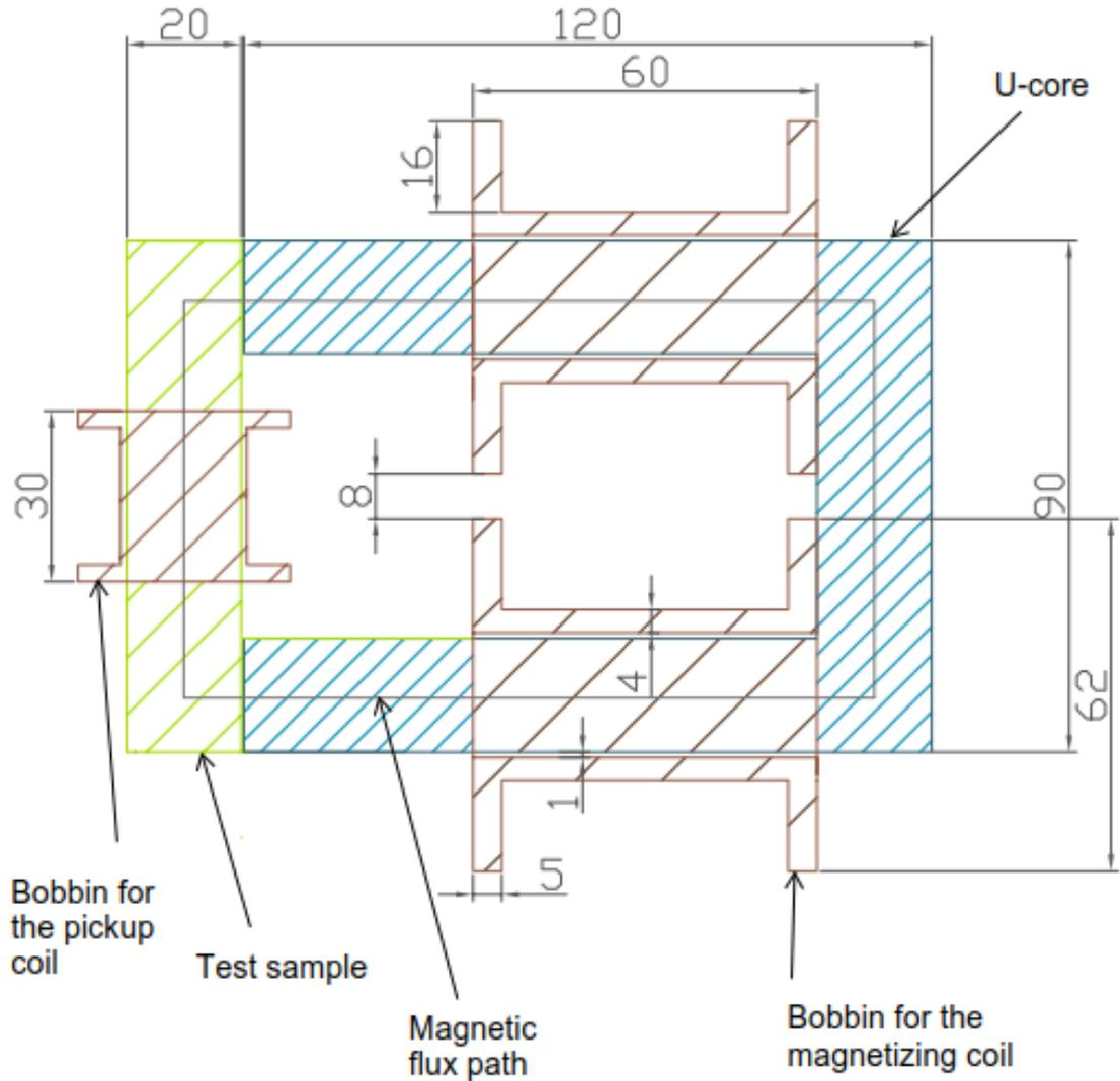
*Figure 4.6: schematic diagram for magnetic circuit.*
