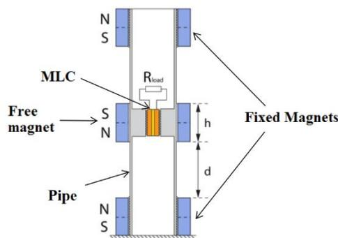
**Figure 2.13:** Structure and working principle of the harvesting device [7].
