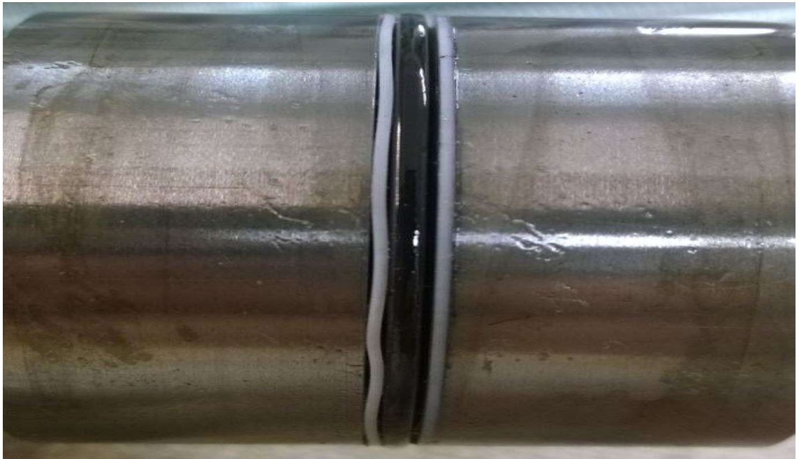
Picture 31 Piston seal 1 from endurance test 2.
