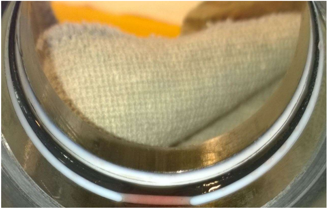
Picture 38 Rod seal 2 from endurance test 2.
