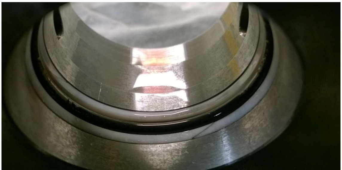
Picture 35 Rod seal 1 from endurance test 1.
