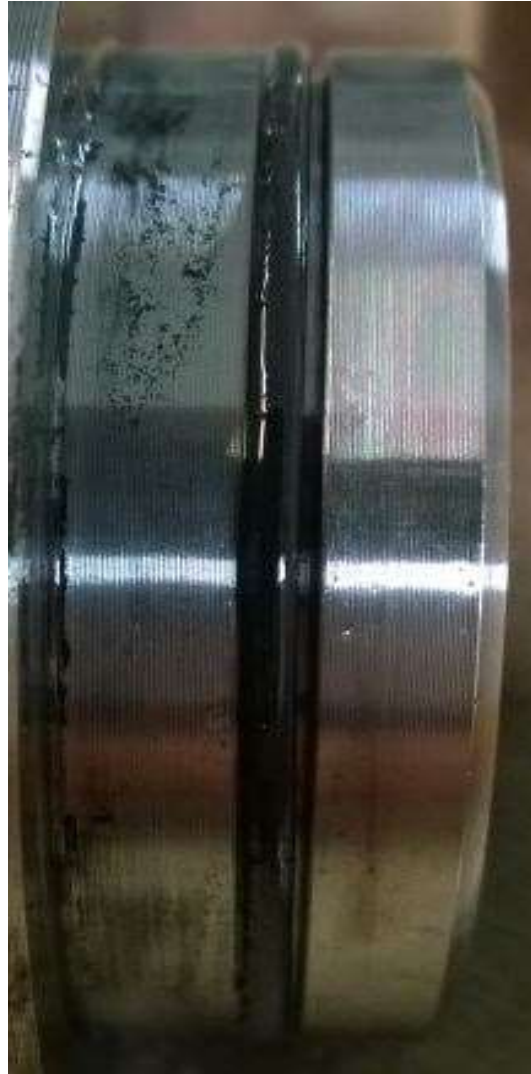
Picture 33 O-ring 2 from endurance test 2.
