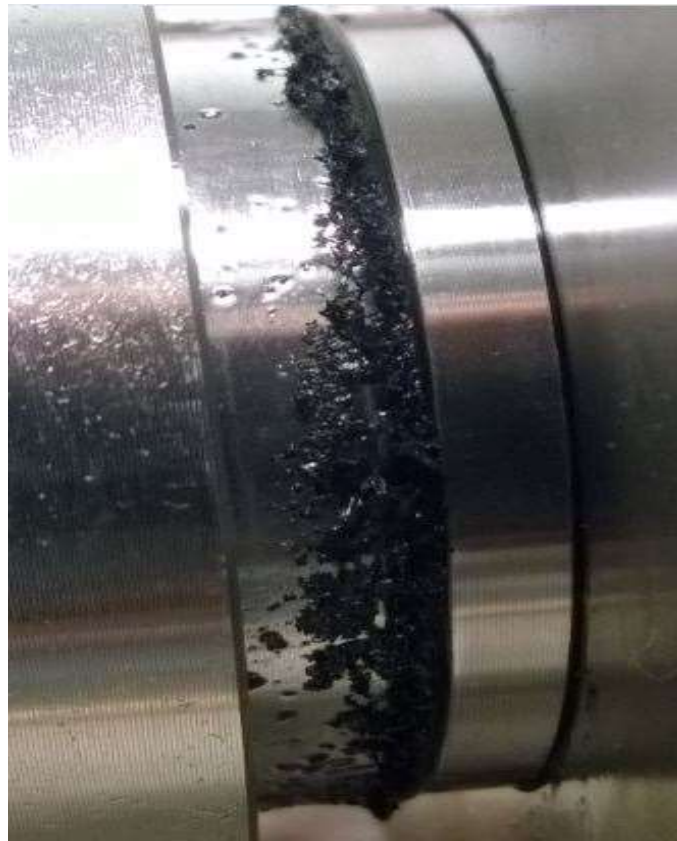
Picture 29 O-ring 2 from endurance test 1.
