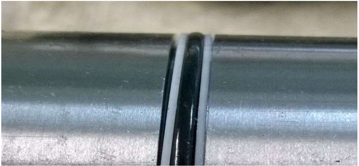
Picture 28 Piston seal 1 from endurance test 1.
