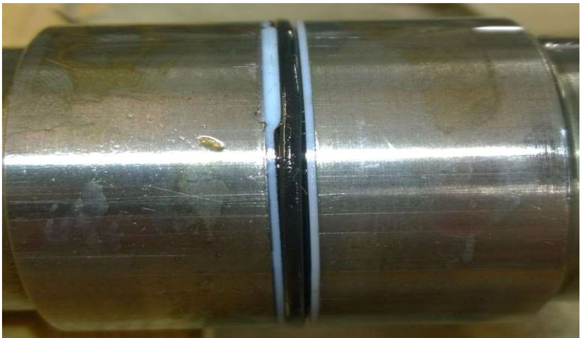
Picture 32 Piston seal 2 from manufacturer 2.
