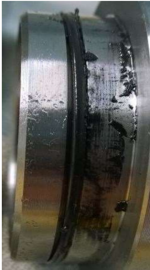
Picture 34 O-ring 1 from endurance test 2.
