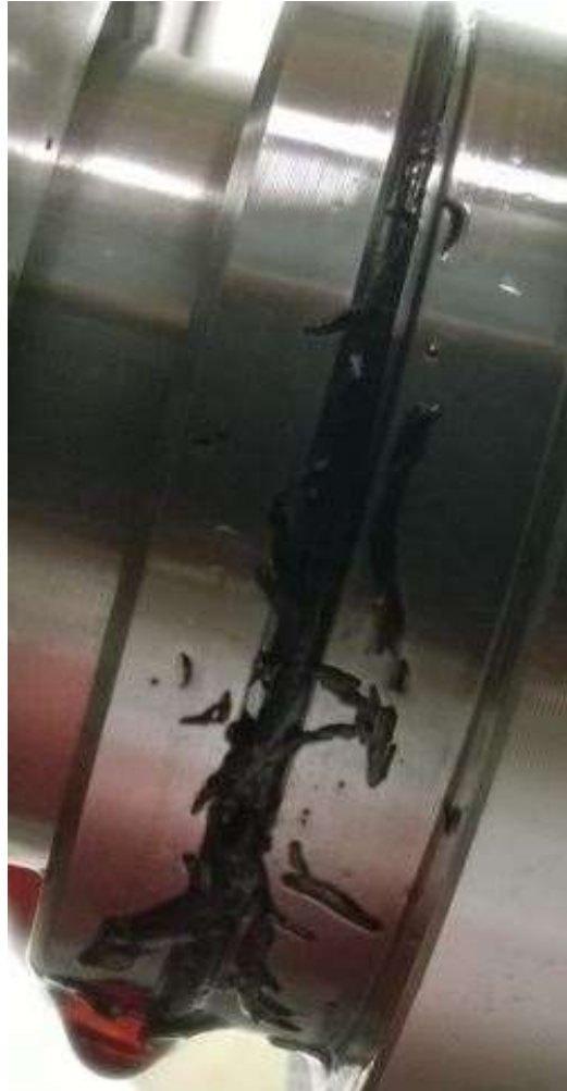
Picture 30 O-ring 1 from endurance test 1.
