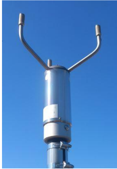
Figure 3.7 WS425 ultrasonic wind sensor.
