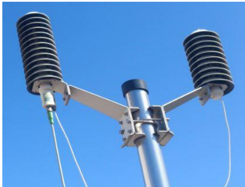
Figure 3.5 HMP155 sensor with the DTR503A and DTR502A radiation shields installed at TUT PV power plant.
