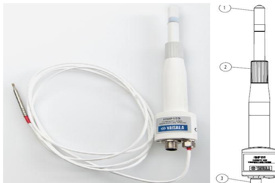
Figure 3.6 HMP155 sensor with structure of the probe (1) Filter (2) Protection cover (3) 8-pin male connector M12 [22].
