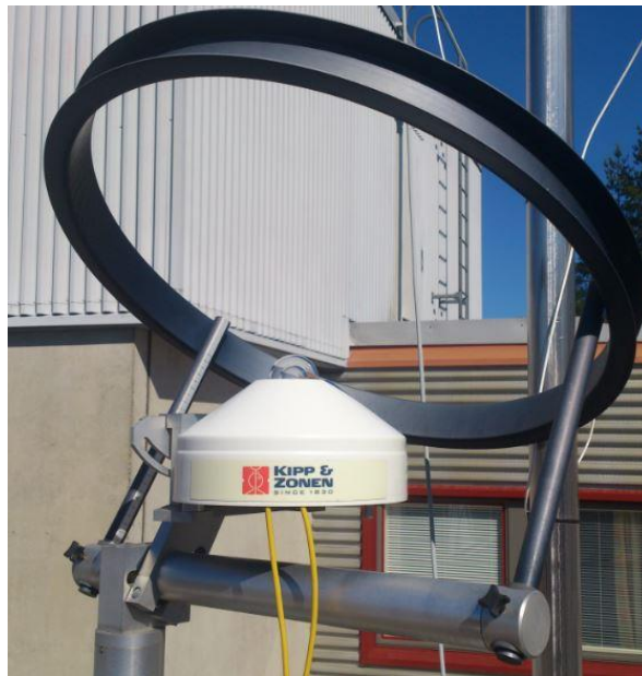
Figure 3.4 CMP21 pyranometer with CM121C shadow ring.
