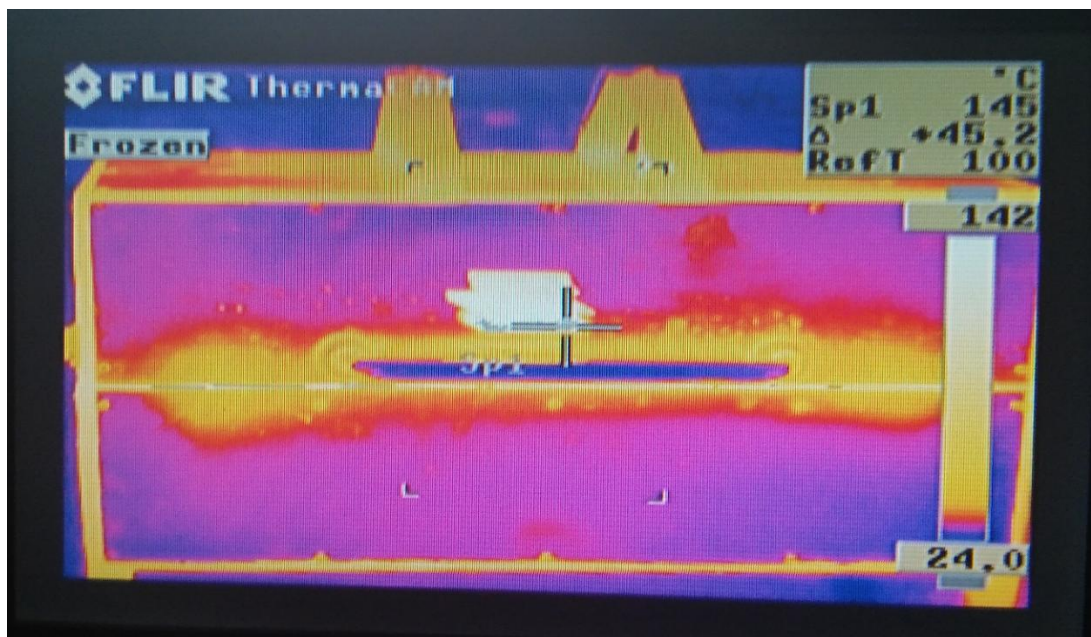
Figure 34. An image taken with the thermal imaging camera from the front of the oven. The white measured area is a black matte surface tape.
