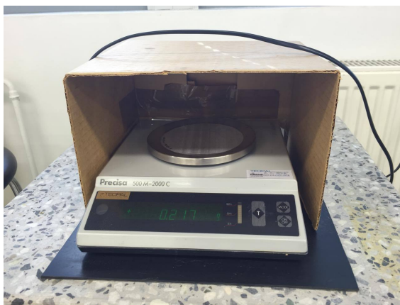
Figure 3.7 Analytical scale, used in weight measurements: Precisa 500M-200C
