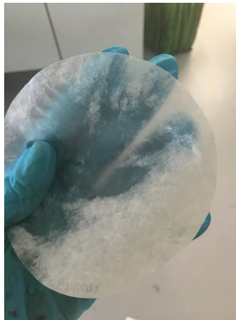
Figure 4.10 Example for variation in adhesion from the level of 3 to 5
