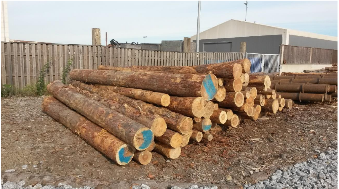
Figure 4.8. Pine logs used in test runs have diameters ranging from 200 mm at top to 500 mm at base. Length for all logs is approximately 5200 mm.
