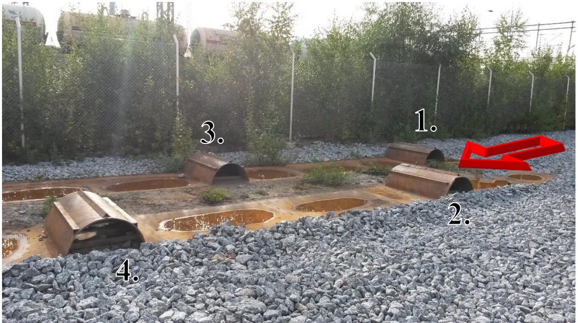
Figure 3.1. Bump track general view. Driving direction shown by red arrow. Bumps are numbered to be referenced later in the results.
