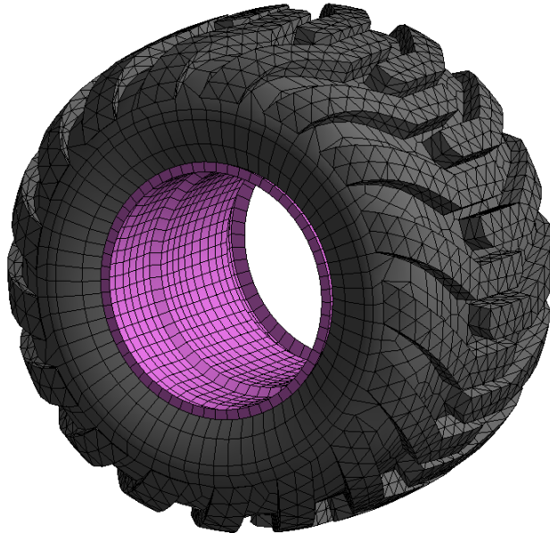
Figure 4.19. Mesh of tire model with solid treads. Nodes of solid and shell tire components are merged.
