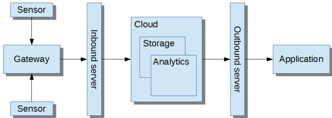
*Figure 9. High-level end-to-end architecture*
