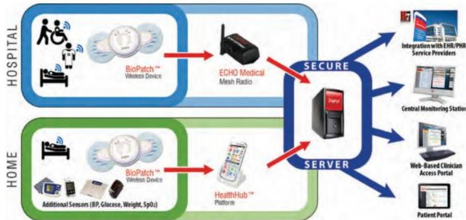
Figure 3. Medtronic remote monitoring system end-to-end architecture. [21]
