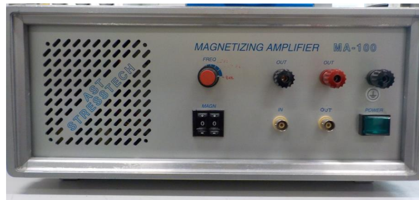
Figure 22 External magnetizing power amplifier MA-100. (Courtesy of Stresstech Oy)
