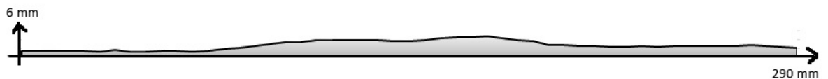
Figure 2 Case depth profile of a hardened steel shaft measured using ultrasonic backscatter technique. [32]
