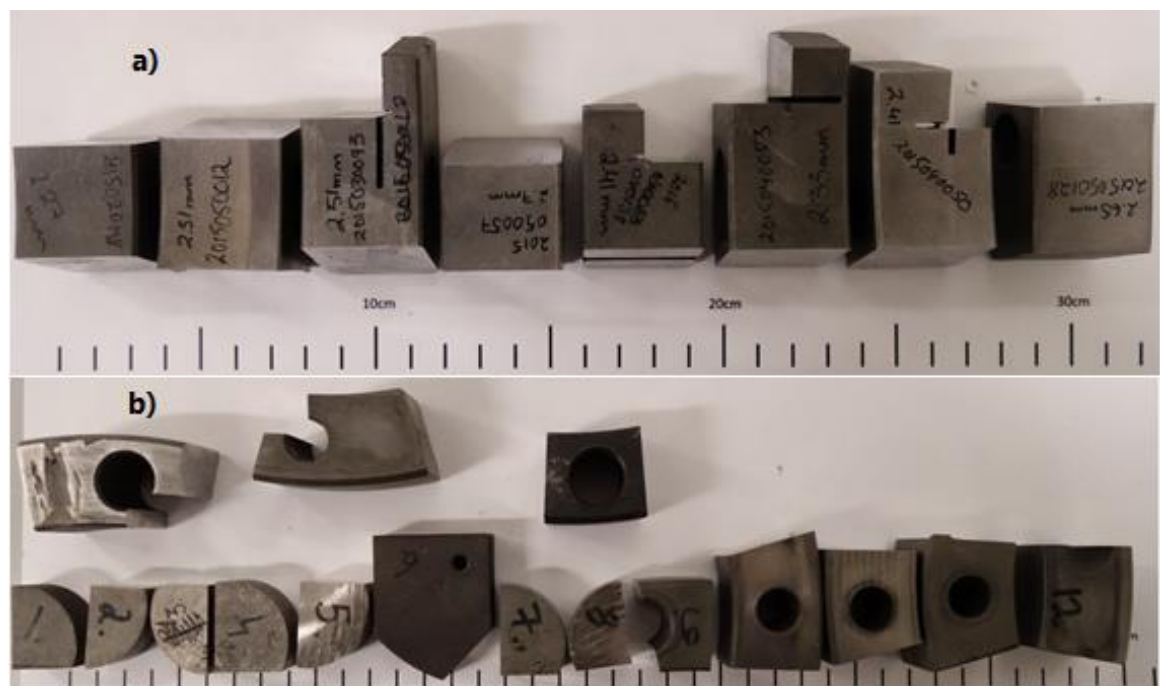
Figure 40 a) The first and b) The second set of case carburized samples.
