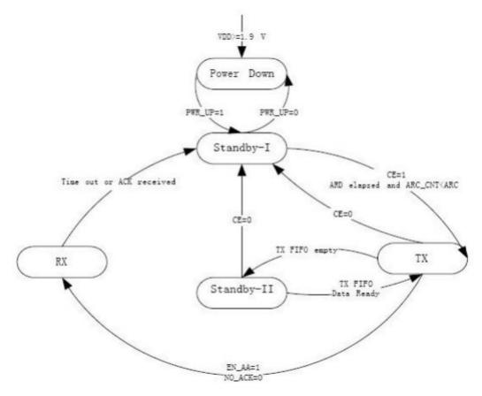
Figure 2.4 RFM73 State Diagram for PTX mode when PRIM\_RX=0 [13]
