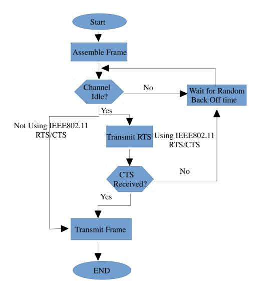
Figure 3.6 Flow Chart Diagram of CSMA/CA protocol Courtesy slidshare.cdn.com
