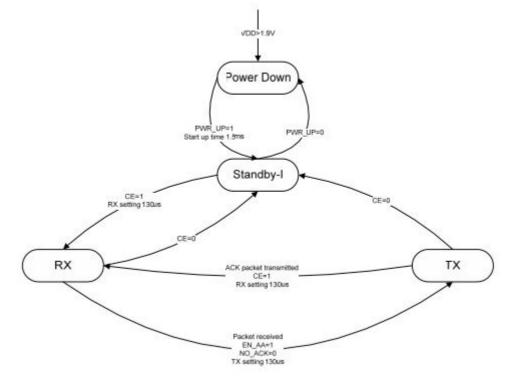
Figure 2.5 RFM73 State Diagram for PRX mode when PRIM\_RX=1 [13]
