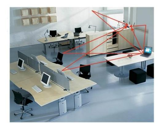
Figure 3.3 Representation of a possible Multipath scenario courtesy to nari.ee.ethz.ch
