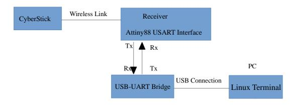
Figure 6.1. Verification Environment for Debugging Messages
