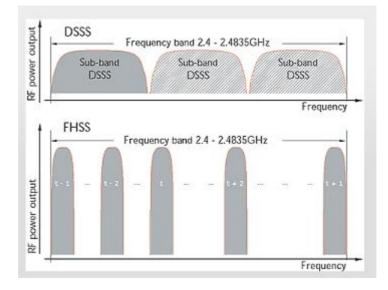
Figure 3.7 Pictorial Representation of DSSS and FHSS courtesy to "Industrial Ethernet" by Bruno Forgue
