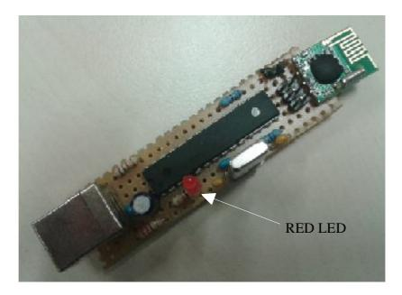
Figure 6.3 RED LED in the Receiver Device
