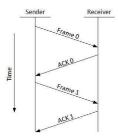
Figure 3.5 ARQ Error Control mechanism courtesy to tutorialspoint.com
