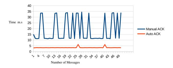
Figure 6.2 Acknowledgement Timing Comparison
