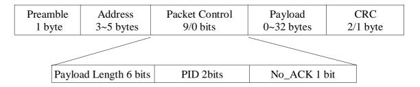
Figure 2.3 RFM Transmission Packet Format [13]
