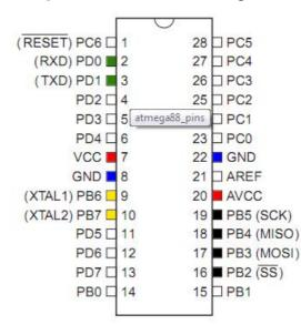
Figure 2.6 Atmega88 pinout courtesy to codeendlife.com
