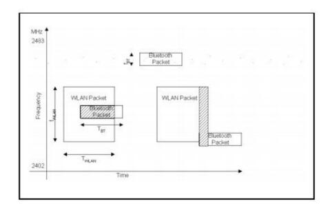
Figure 3.1 Time and Frequency Collisions in the 2.4 Ghz ISM band [22]
