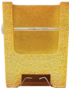
Figure 2.17 Cross-section of a disposable CCA sample cup [34].
