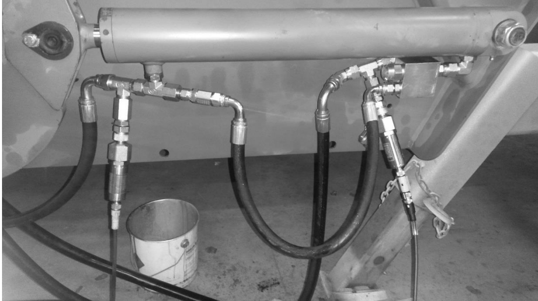
Figure 52: Pressure sensors for pilot and back pressures
