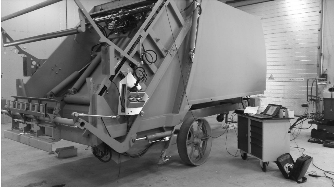
Figure 50: The compactor and the testing equipment used in the binlift measurements
