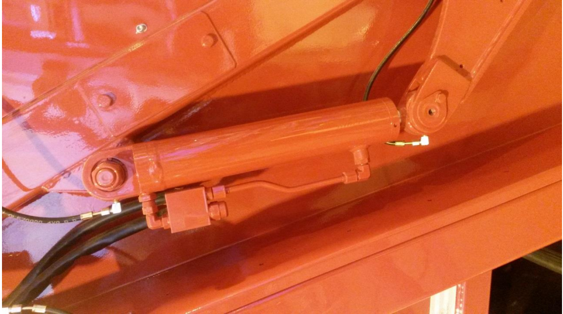
Figure 43: Installation of the cartridge valve on the cylinder
