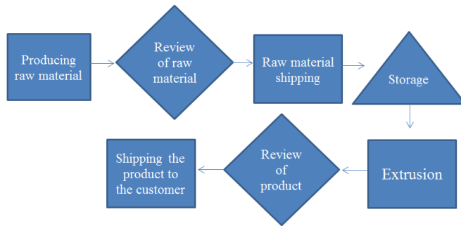
Figure 3 A very simple macro flowchart of plastic extrusion process, a box = an activity, a diamond = a review, an arrow = the direction of the flow, a triangle = a storage, the big D (not in the figure) = delay (adapted from Madison 2005, p. 19-21)
