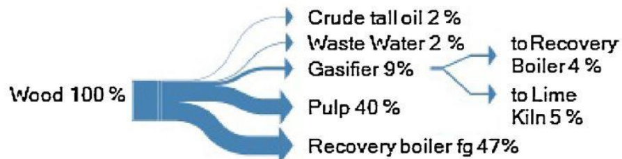
Figure 3. Carbon flows in a modern pulp and paper mill. Adapted with permission. [43]
