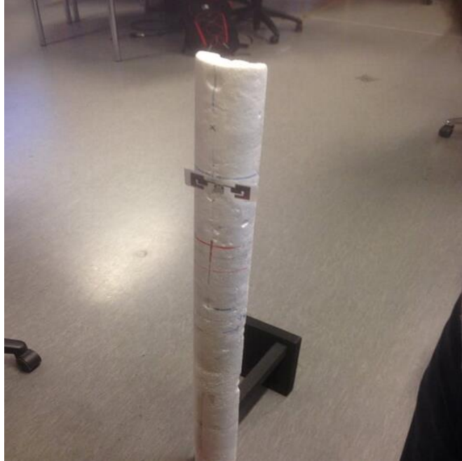
Figure 6-8 Thermophore Stand for Placing RFID Tag
