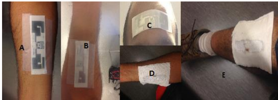
Figure 6-1 Different RFID Tags Placement While Taking Measurements (A) Dogbone Tag placed on Hairy Side of Arm (B) Dogbone Tag Placed on Non-Hairy Side of Arm (C) Dogbone Tag Placed on Forehead (D) Tag on Rayon Bandage Placed on Non-Hairy Side of Arm (E) Tag on Rayon Bandage Placed on Front Side of Leg
