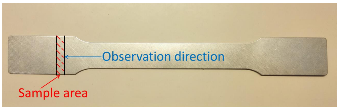
Figure 25. Schematics of the sample area on the tensile specimen for microstructure observation
