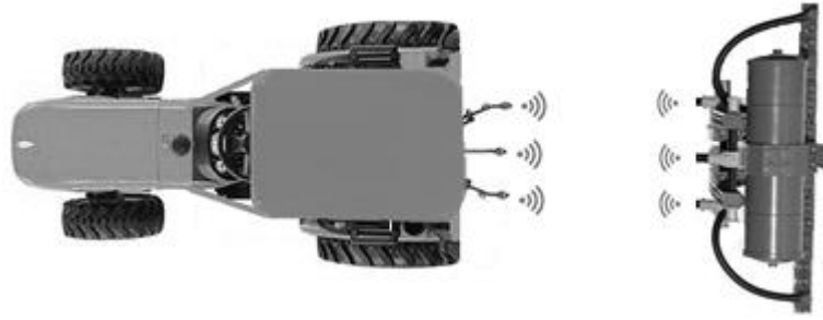
Figure 55. Demonstration of automatic coupling of tractor implement.
