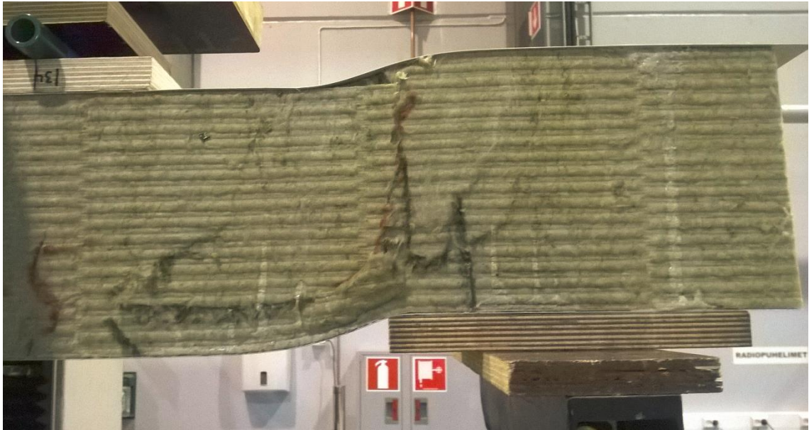
Figure 40: Test specimen with shear failure
