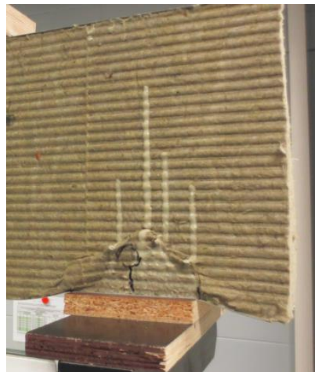
Figure 36: Crushing failure on the support with the thicker test specimen
