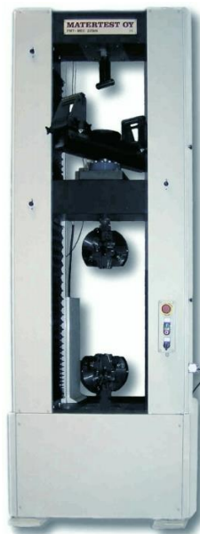
Figure 29: FMT-MEC material testing machine (Matertest Oy)
