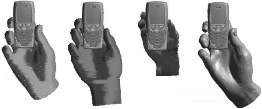
Figure 6. Hand models (from left to right) in the order from Grip 1 to 4. Aligned using the Nokia 8310 phone model as reference. [37]
