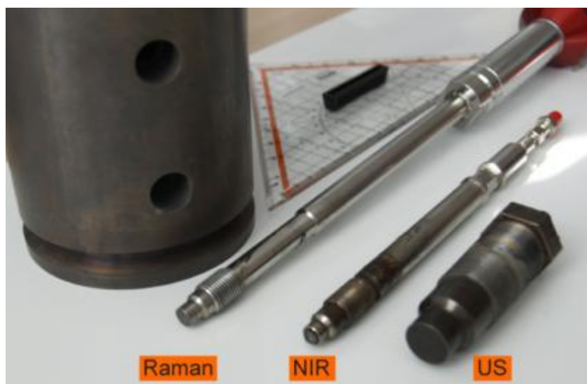
Figure 5.2. Raman, Near Infrared (NIR) and ultrasonic (US) sensors. A measurement slit die is partially shown on the left side. Modified from (Alig et al. 2010).
