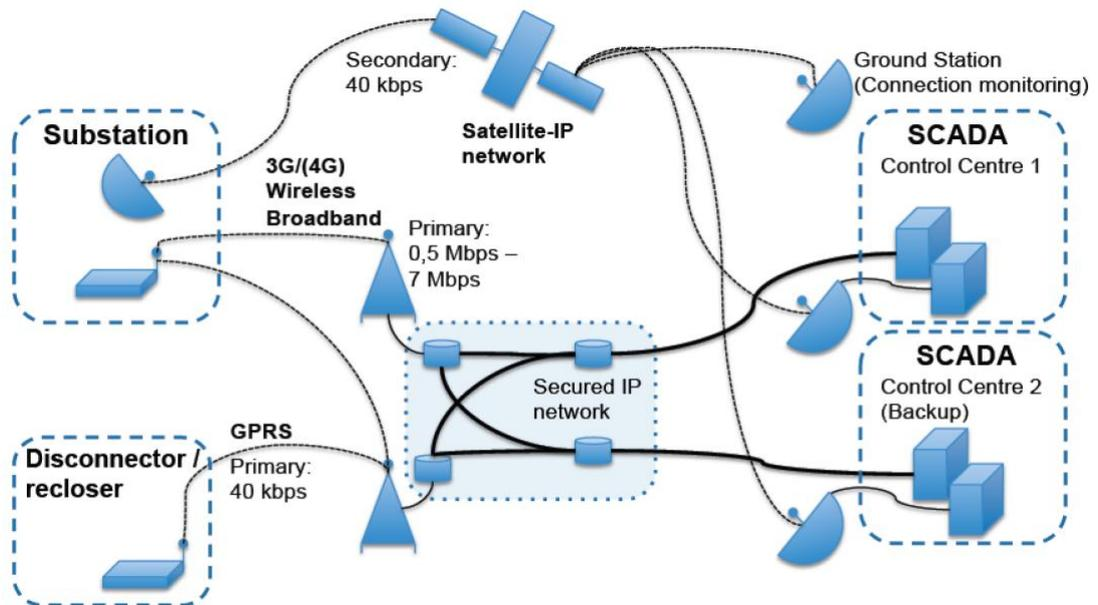
*Figure 4-6: Field communication system used by Elenia (Verho, 2013)*
