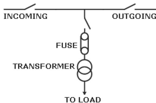
*Figure 3-2: Basic RMU unit for SS*
