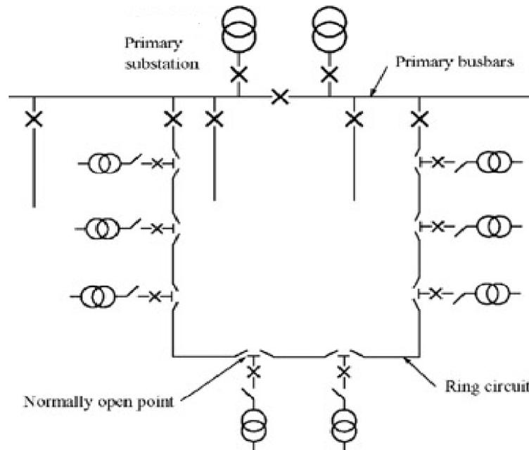
*Figure 3-1: MV network in ring mains configuration*
