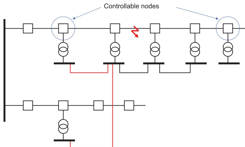
**Figure 4-3: LV coupling beneath the RMU configured MV network**
