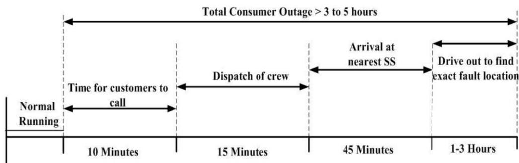
*Figure 3-3: Fault Management timescale (without FLISR process)*
