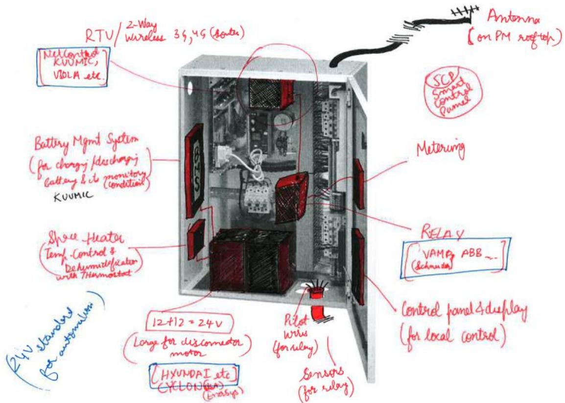
*Figure 5-6: Initial sketch for SN Panel*
