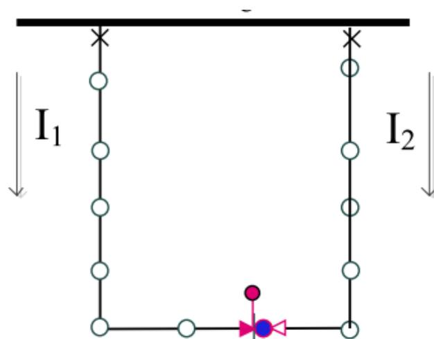
*Figure 3-6: MV-distribution RMU configured enabling shift of NOP [28]*
