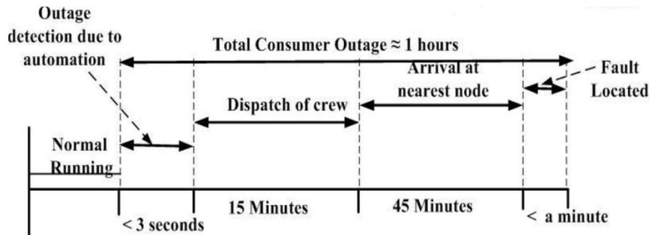
*Figure 3-4: Fault Management timescale (with FLISR process)*
