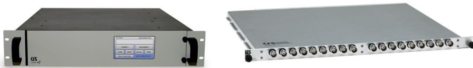
Figure 3.6 G2 series switching system and mainframe [24]
