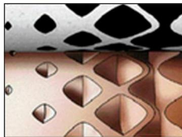
**Figure 3.5** Pixelated ink transfer from the gravure cups onto the substrate [21].
