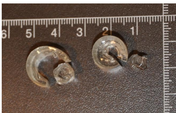
Figure 20. Two gelatin-siloxane test pieces after fracture. Left: 15G10G Right: 15G15S.
