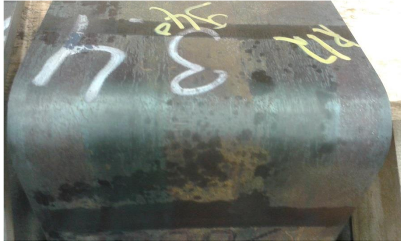
Figure 65: Illustration of a sample containing stripes of red scale.
