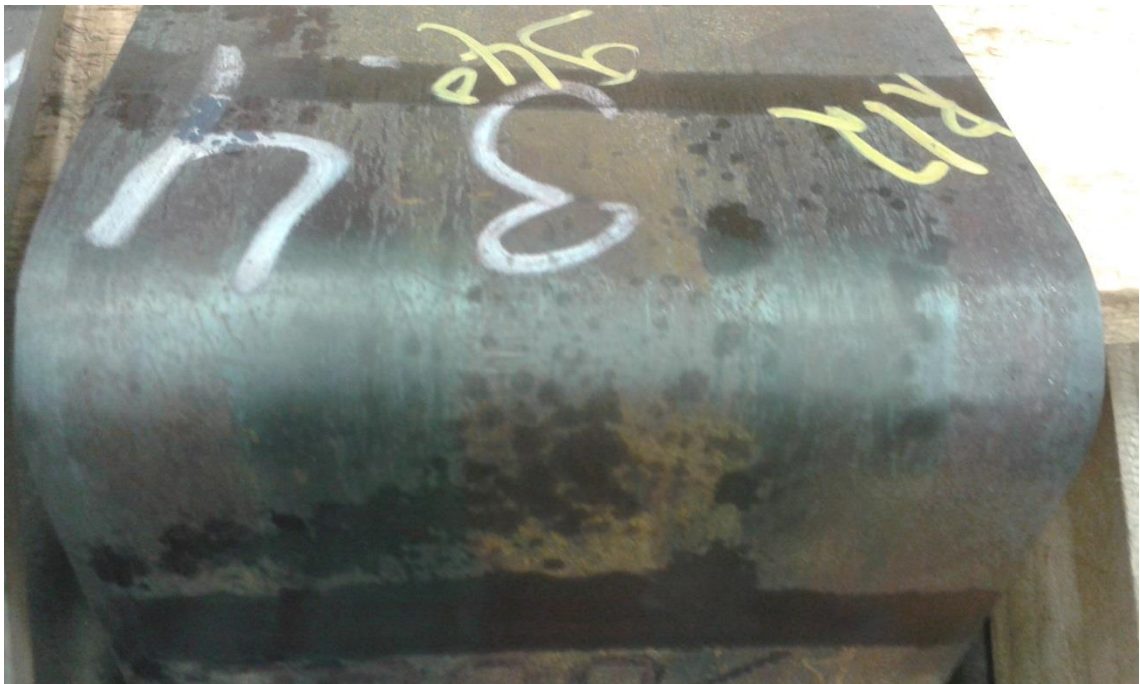
Figure 83: Sample 0.07C-1.3Mn 815°C bent to an angle of 94°.
