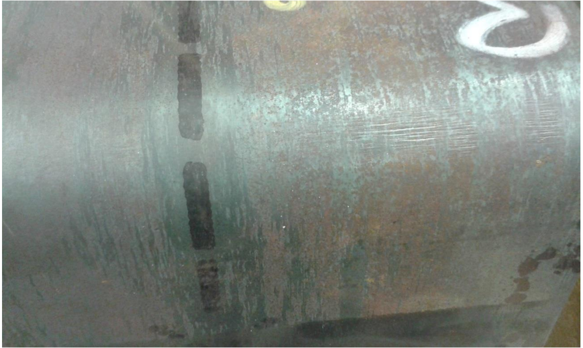
Figure 76: Damage occurring at the surface of the bent sample in regions containing red scale.
