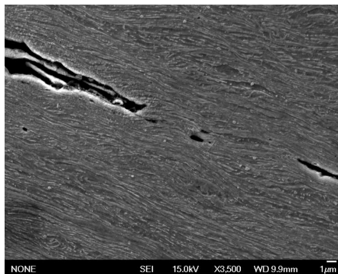
Figure 79: The lower part of the fracture at the depth of 0.4 and shear bands.
