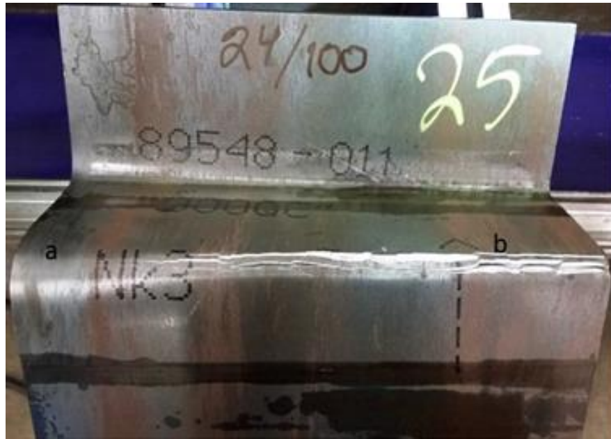
Figure 60: Sample 0.08C-1.8Mn 815°C a) no visually observable damage and b) visually observable damage at the surface.
