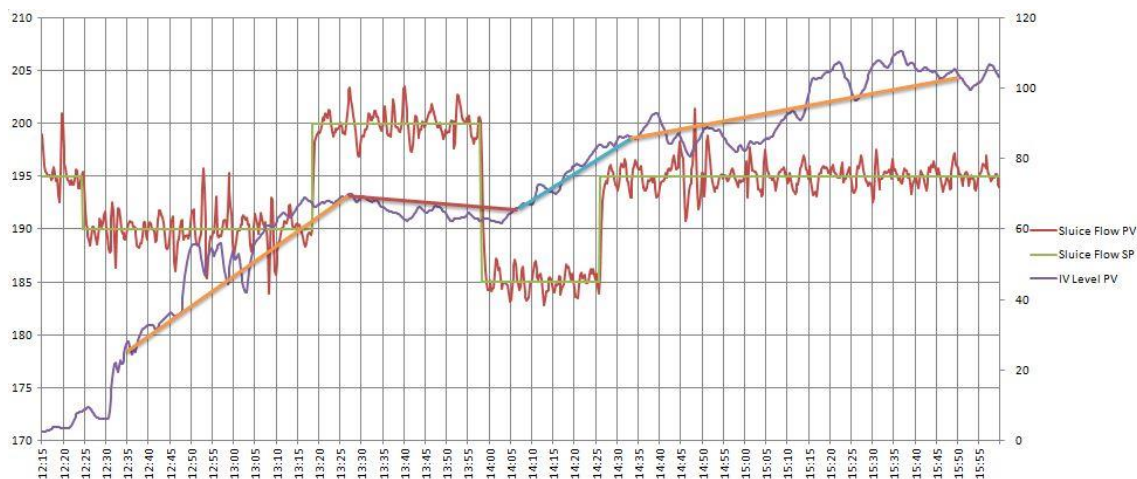
Figure 23: Fitting slopes to step response data. Red curve indicates sluice flow process value, green curve indicates sluice flow setpoint value, and magenta curve indicates IV level process value.
