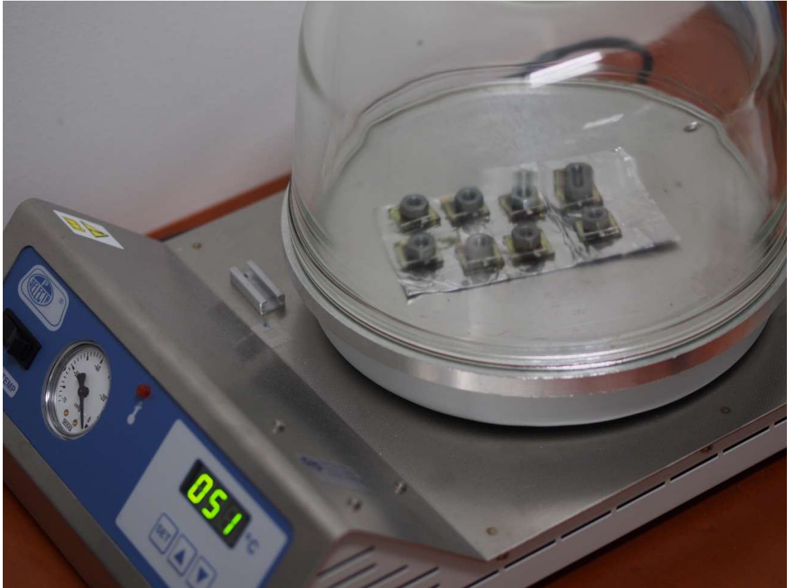
Figure 3.2. Solar cells being sealed.
